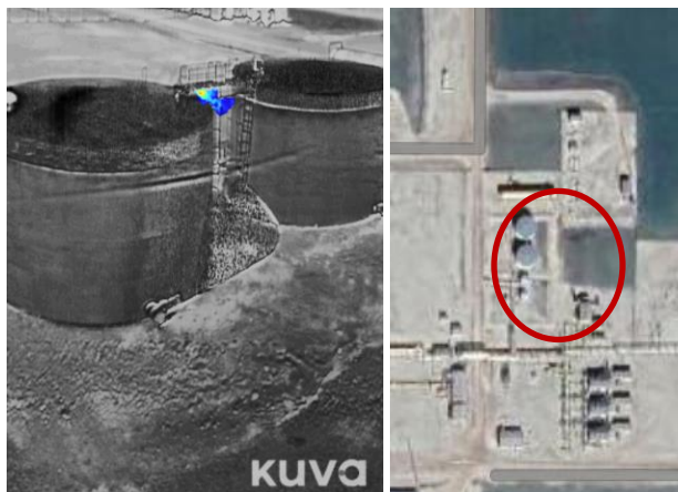
Figure 20: Baseline emission detection with Kuva™ from south tank (TK-101A)
