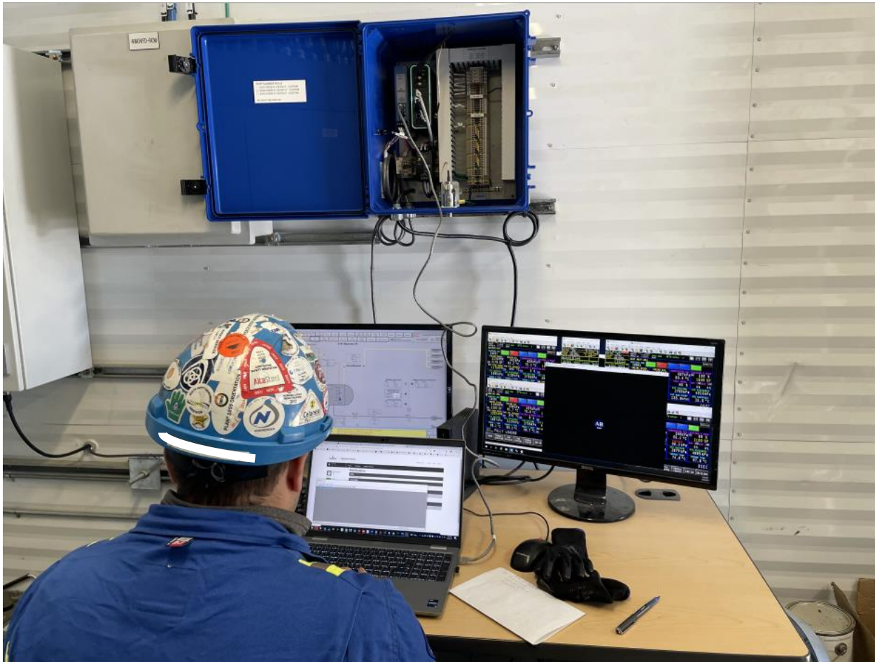
Figure 11: Local and remote data acquisition through wireless gateway
