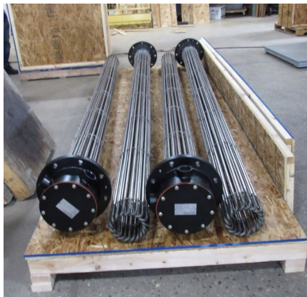
Figure 6: Production Tank Heaters
