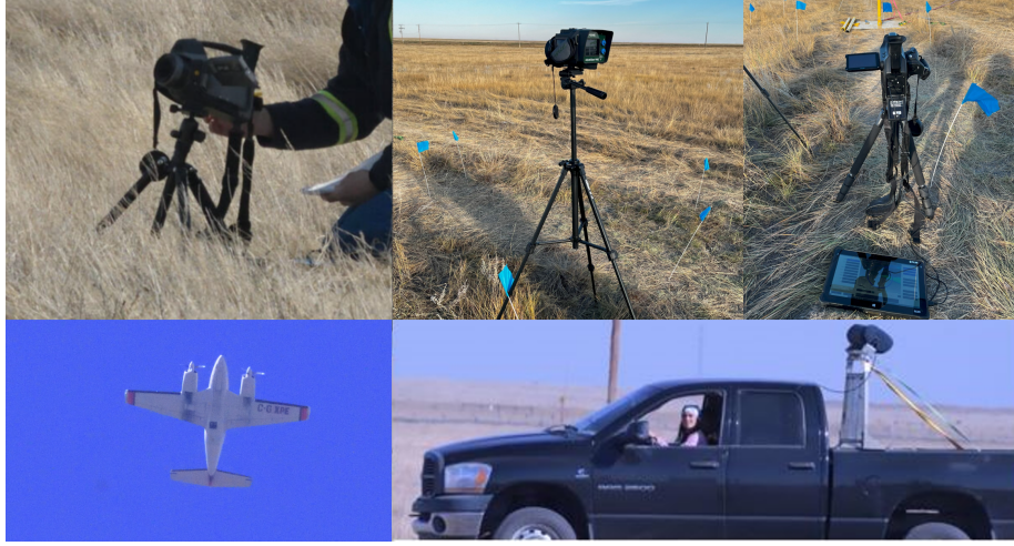
Figure 1: Technologies studied in the field trials. Top row, left to right: QOGI A, QOGI B, QOGI C. Bottom row, left to right: airborne NIR HSI, truck-based TDLAS.
