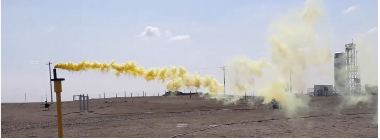
Figure 19: Instantaneous snapshot of tracer smoke from the first field campaign, highlighting that the instantaneous concentration field differs from the time-averaged profile, even under constant wind conditions.
