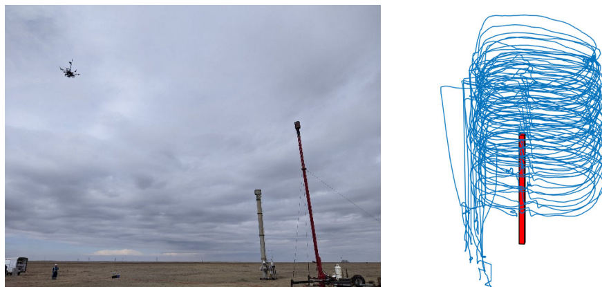
Figure 3: Example helical path flown by the TDLAS-equipped drone in the first field campaign.
