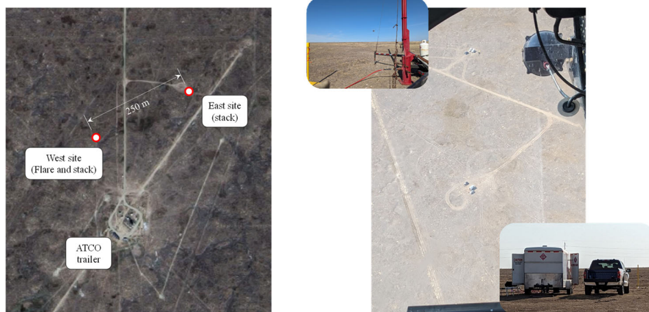
Figure 9: Location of releases for the third field trial, and view from the LSI helicopter. The helicopter flew repeated east-west and west-east passes, with pauses of 2-3 minutes each time the release rate was changed to allow the plume to develop.
