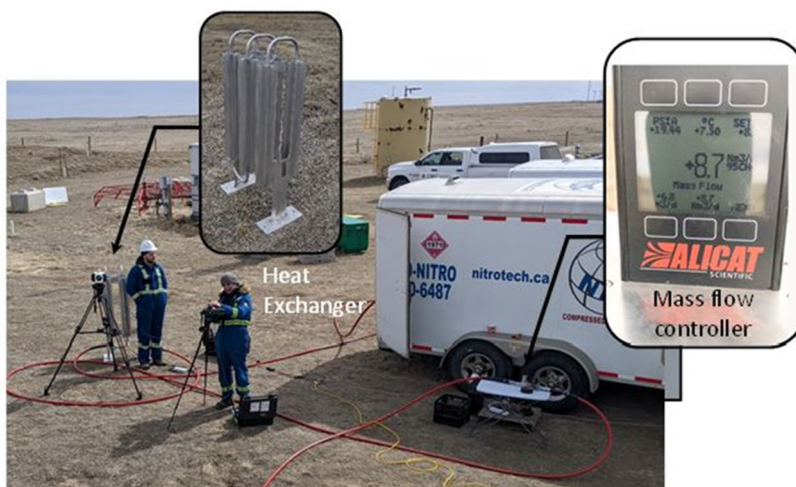
Figure 8: Compressed gas was released via a regulator and then conditioned to the ambient air temperature using a heat exchanger, before entering the mass flow controller. It was subsequently discharged to the atmosphere according to the particular release condition.
