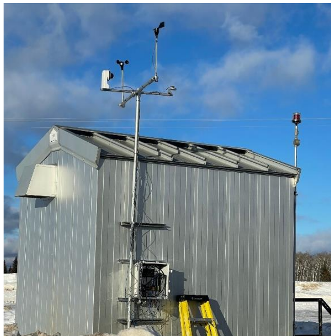
Figure 5 – SRC Weather Station (Please refer the top-right part of Figure 2)
