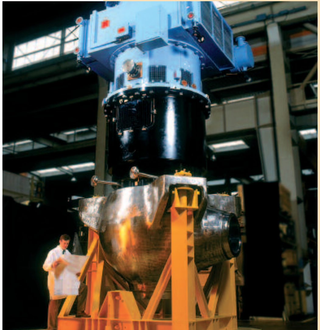
Jeumont manufacturing plant (France): reactor coolant pump (N4,1,500 MWe).
