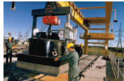
Figure 6-2 MACSTOR Fuel Transfer
