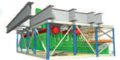
Heat Transport System Upper Header Module with Pipe Whip Restraint
