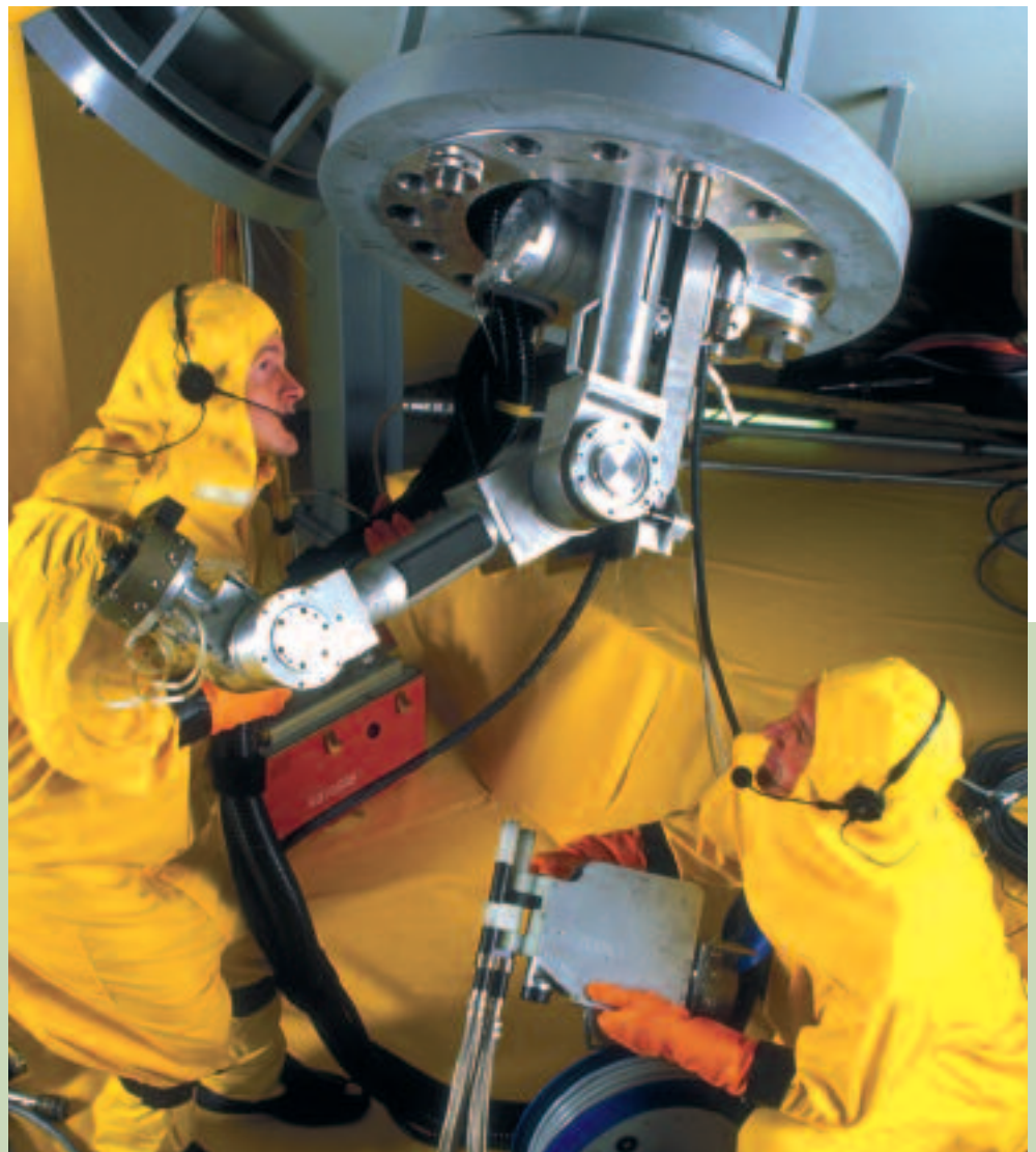
Lynchburg technical center (Va, USA): training for steam generator inspection.
