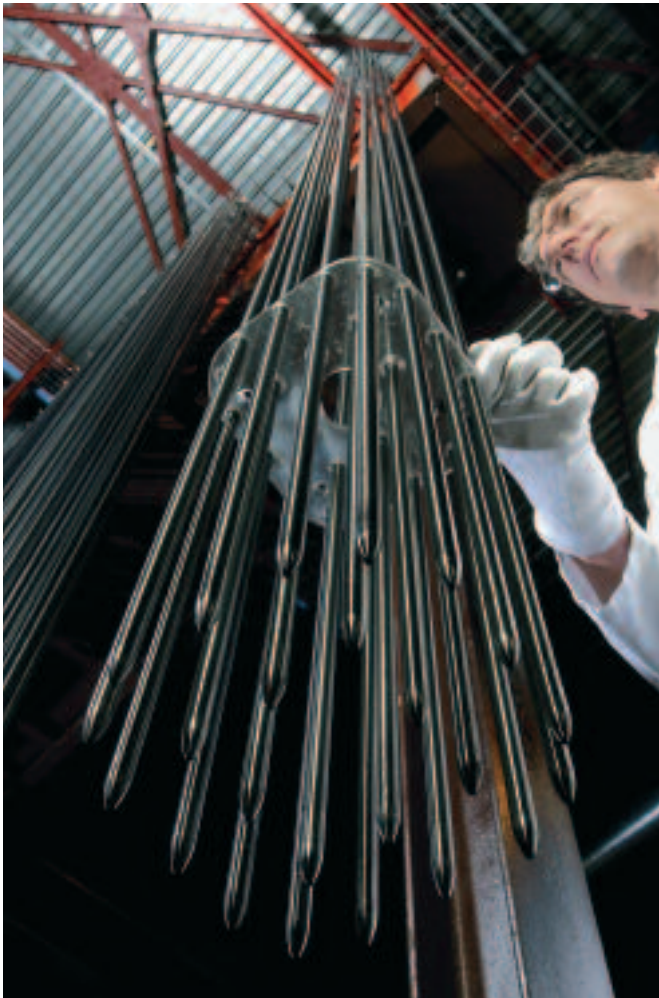
RCCA manufacturing at the FBFC Pierrelatte (France) fuel fabrication plant.
