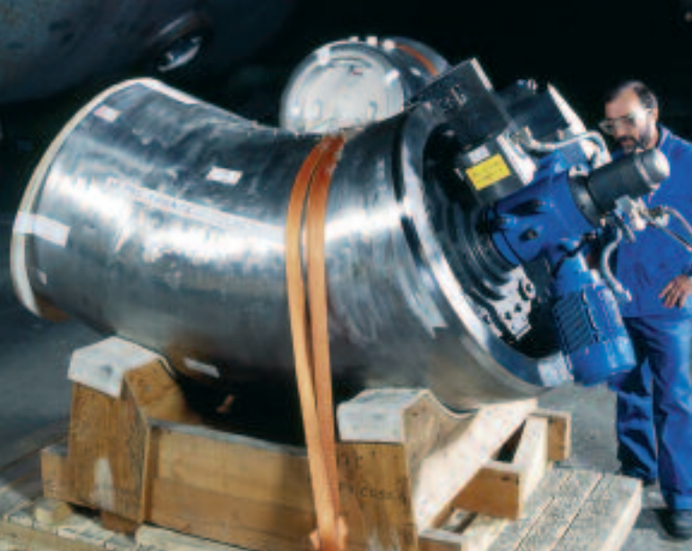
Chalon manufacturing plant (France): machining of primary piping elbow.
