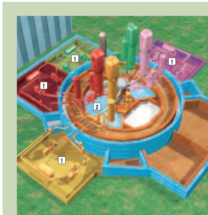
The major safety systems comprise four sub-systems or trains, each capable of performing the entire safety function on its own. There is one train in each of the four safeguard buildings (1) surrounding the reactor building (2) to prevent a simultaneous failure of the trains.
