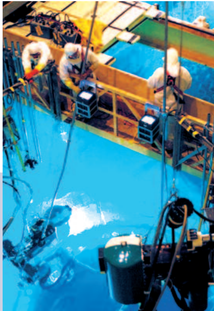
In-service inspection machine for ultrasonic testing of reactor pressure vessels.
