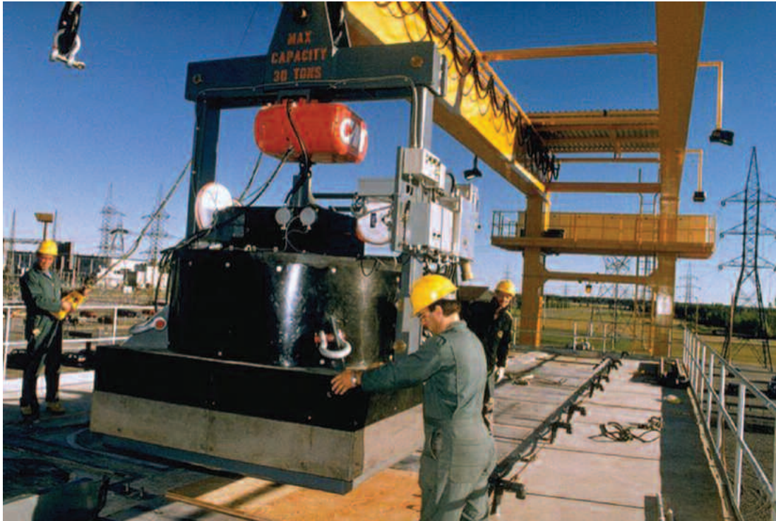
Figure 6-2 MACSTOR Fuel Transfer
