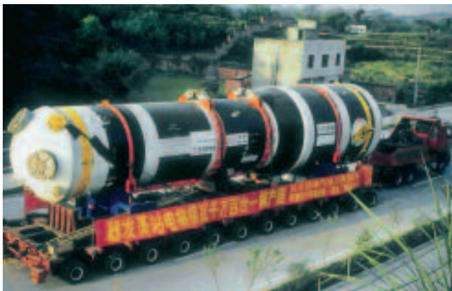
Transportation of a steam generator manufactured in China for Ling-Ao 2.
