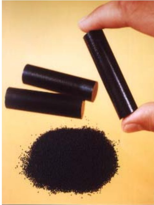
Figure A-10, TRISO Particles & Compacts (GA)
