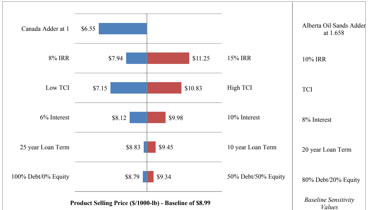
Figure 15. Effect of variations in key economic parameters on the price of steam.
