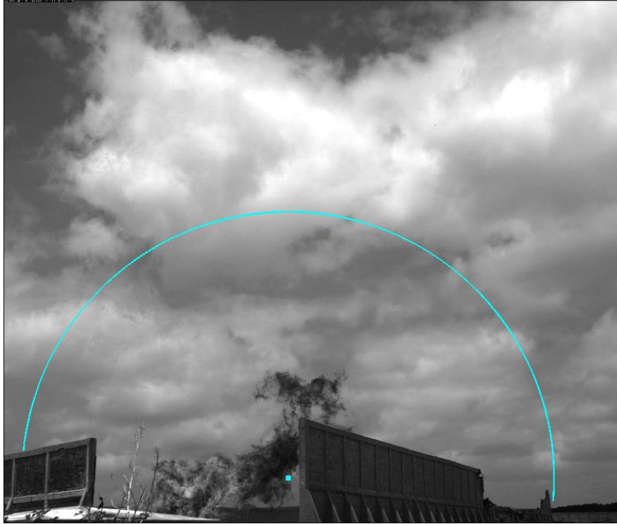
Figure 5: Sample grayscale image of the horizontal pit flare acquired using the sky-LOSA acquisition system with the control surface defining the instantaneous BC emission rate superimposed.
