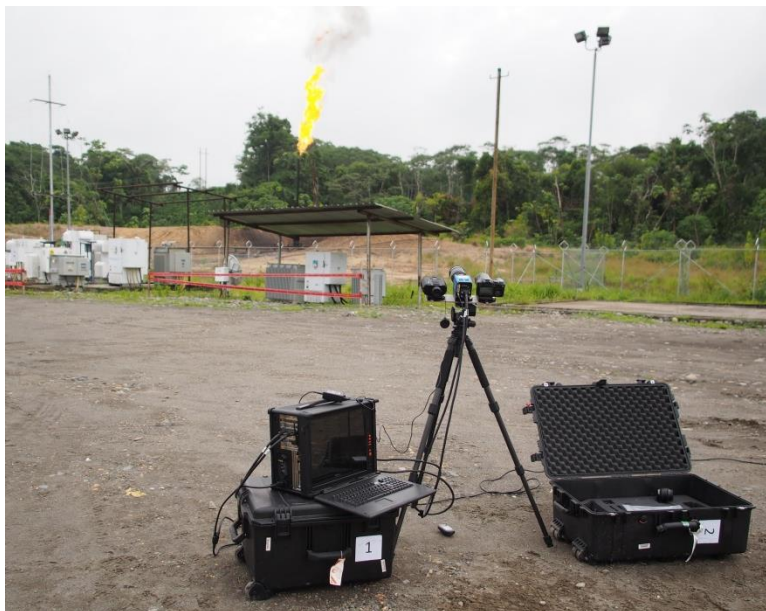
Figure B.4: Sky-LOSA setup at Auca 27. From left to right - rugged portable field computer, tripod with laser rangefinder, sCMOS camera, and consumer-grade video camera, and case for additional lenses and optical filters as necessary during measurements. The system is powered through an inverter connected to the battery system of a nearby vehicle located to the right of the image.
