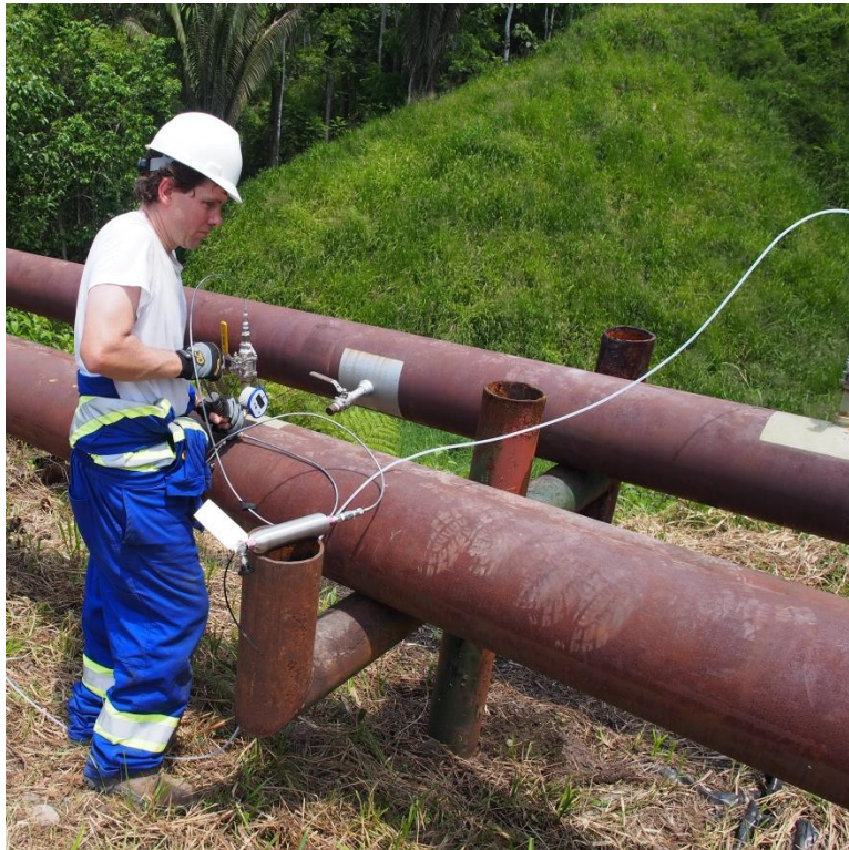
Figure B.10: Filling a sample cylinder from a hot tap with hand pump at Auca Sur.
