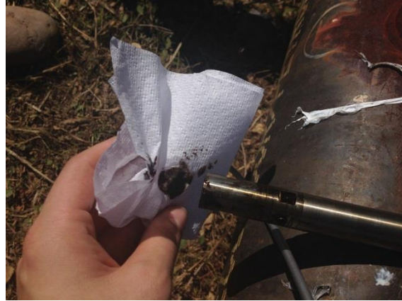
Figure B.16: Solids in bottom of Line 3 at Auca Sur 1 on OFM probe.
