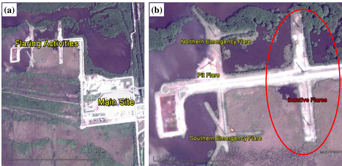
Figure 2: Flaring infrastructure at the Atasta Compressor Station. a) the location of flaring activities with respect to the main site and b) the locations of active flares. The three easternmost flares were not in use during measurements as construction work was being performed. To the west were two stack flares composing the emergency system and a single horizontal pit flare composing the compressor purge system.
