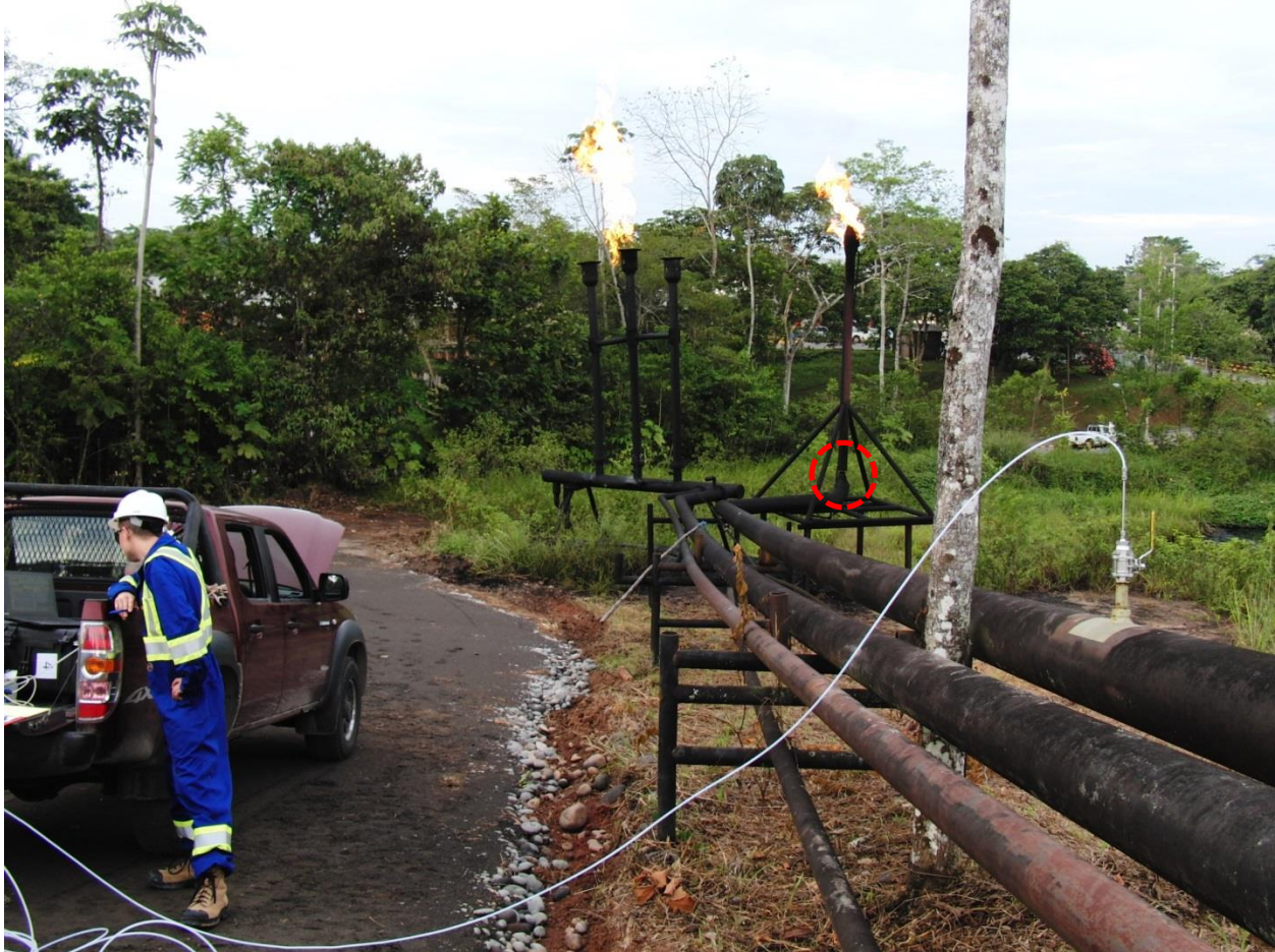
Figure B.11: Flare setup at Auca Central with the Venturi air-entrainment circled in red.
