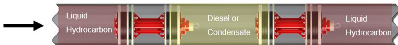
Figure 3. In-Service Initial Cleaning for Liquid Pipelines
