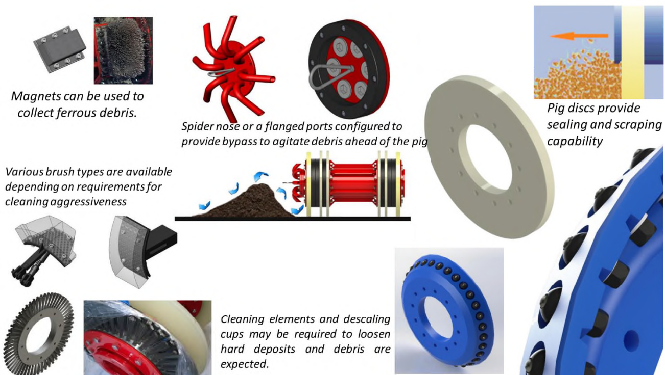
Figure 12. Examples of cleaning elements of varying aggressiveness that may be incorporated with mechanical pigs and considered for Phase 2 of a progressive cleaning program
