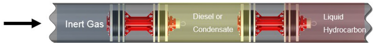
Figure 7. Diagram of the displacement and cleaning stages recommended for liquid lines
