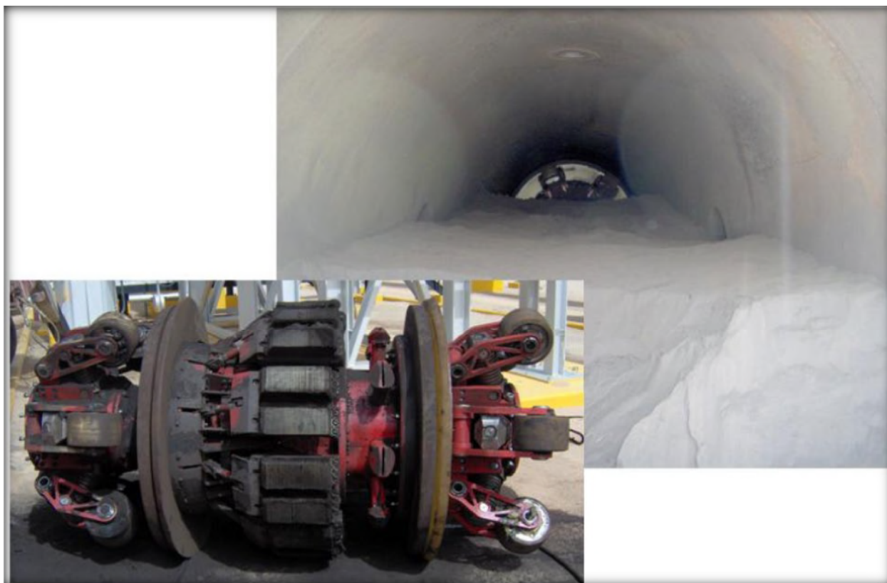
Figure 14. Receiver filled with black powder and Cleaning tool after a 170-km run in a pipeline
