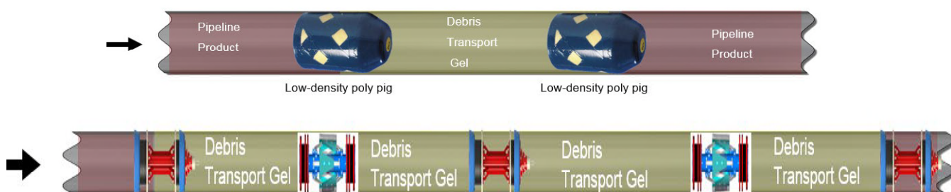
Figure 8. Example of pipeline gel-cleaning program involving poly pigs followed by more aggressive cup/disc pigs.
