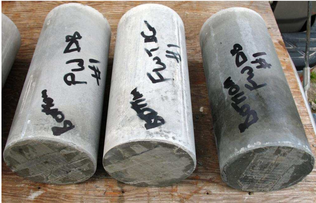
Bottom View Of Tubing Placed (Labelled TBG) & Dump Bailed (Labelled DB) Samples
