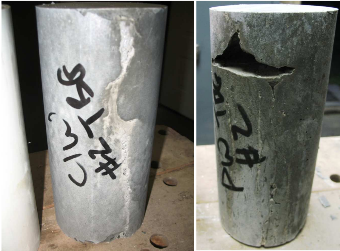
Tubing Placement In Corrosion Inhibited And Produced Water Showing Voids Along Side. Cut From Samples 860 to 1075 mm From Bottom Of Test Sample (Near Top Of Sample)
