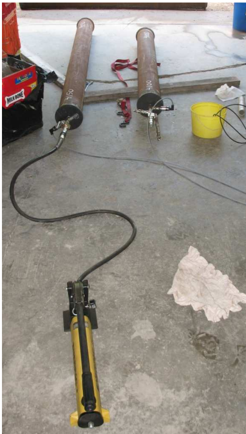
Pressure Test Apparatus Prior To Extending And Securing Hose Sample 4100 Leaking During Test
