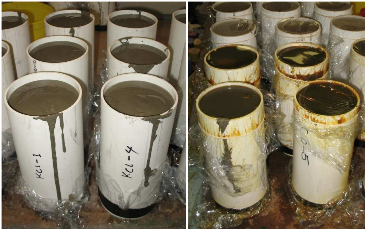
Compression Test Samples Poured & Then Topped With Fluid & Sealed
