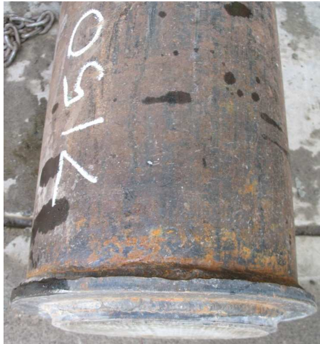
Sample 7150 With 2.0 mm Plug Movement
