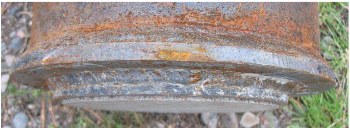
Sample 7150 With 2.0 mm Plug Movement
