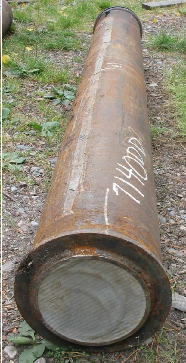
Sample 7140DD Cement Plug End
