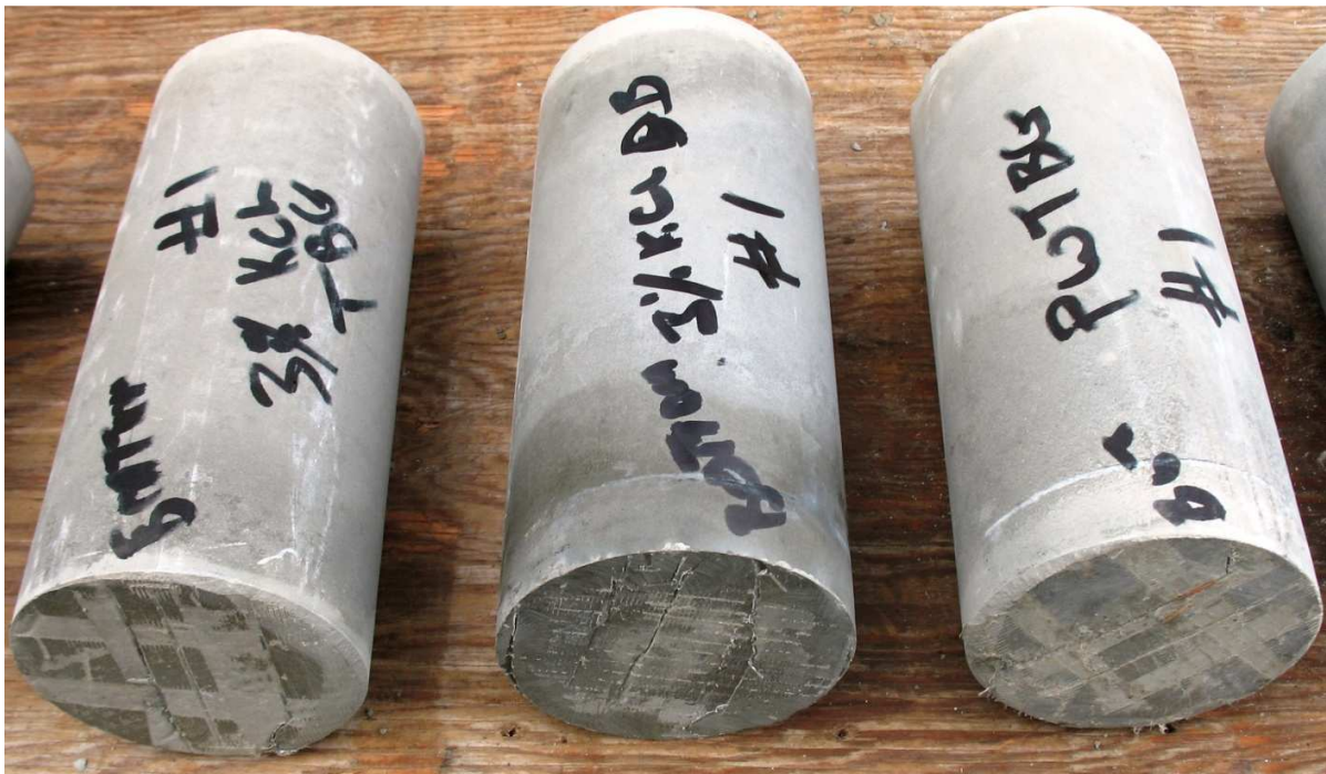
Bottom View Of Tubing Placed (Labelled TBG) & Dump Bailed (Labelled DB) Samples
