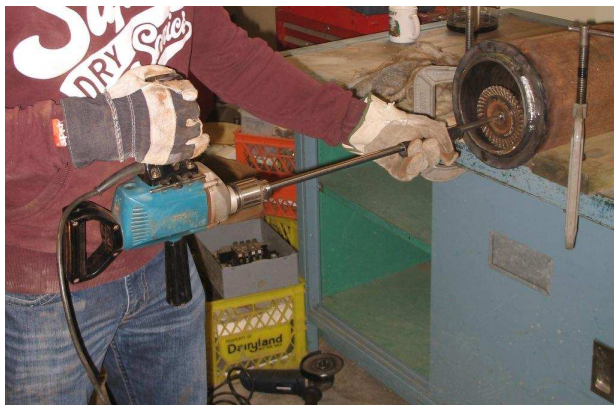
Cleaning Pipe Surface Prior To Cementing
