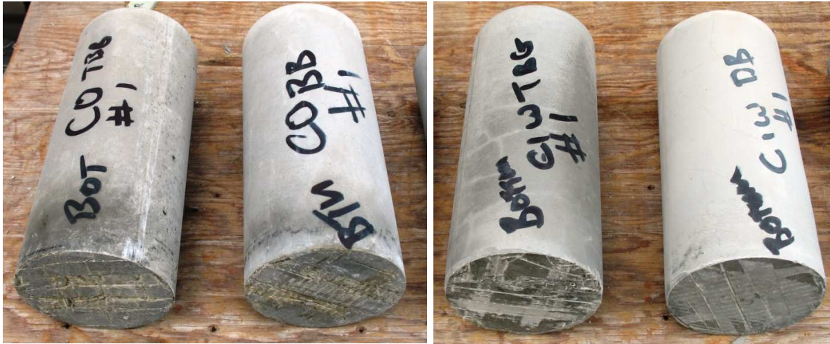
Bottom View Of Tubing Placed (Labelled TBG) & Dump Bailed (Labelled DB) Samples
