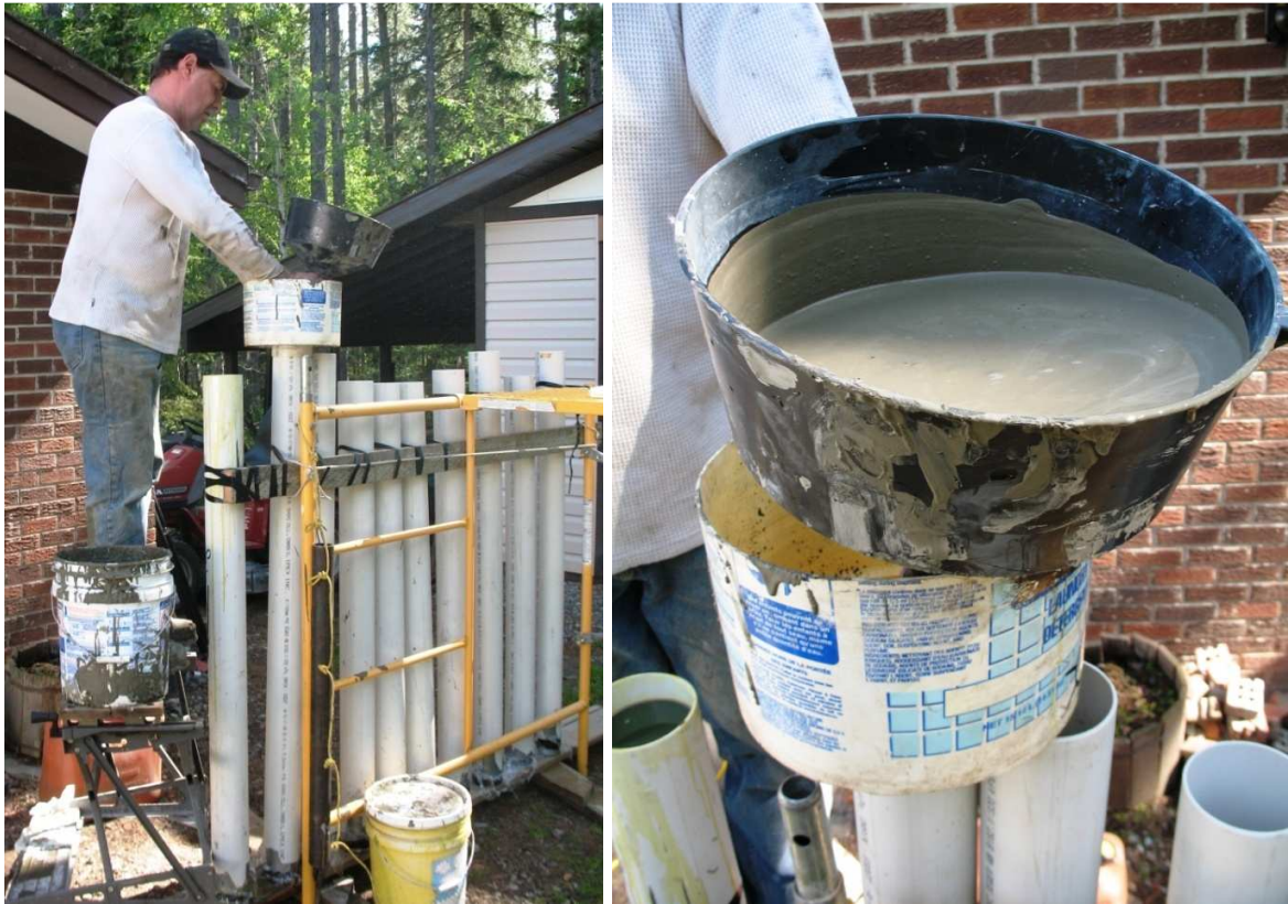
Compression Test Samples – Placing Cement With Funnel And Hose (Tubing Placement)
