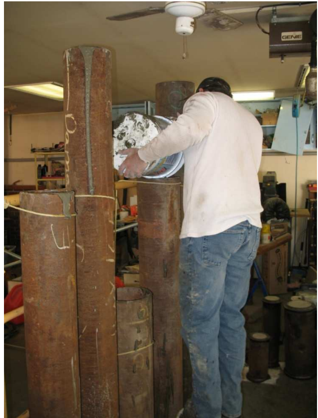
Pouring Cement In Pressure Test Samples
