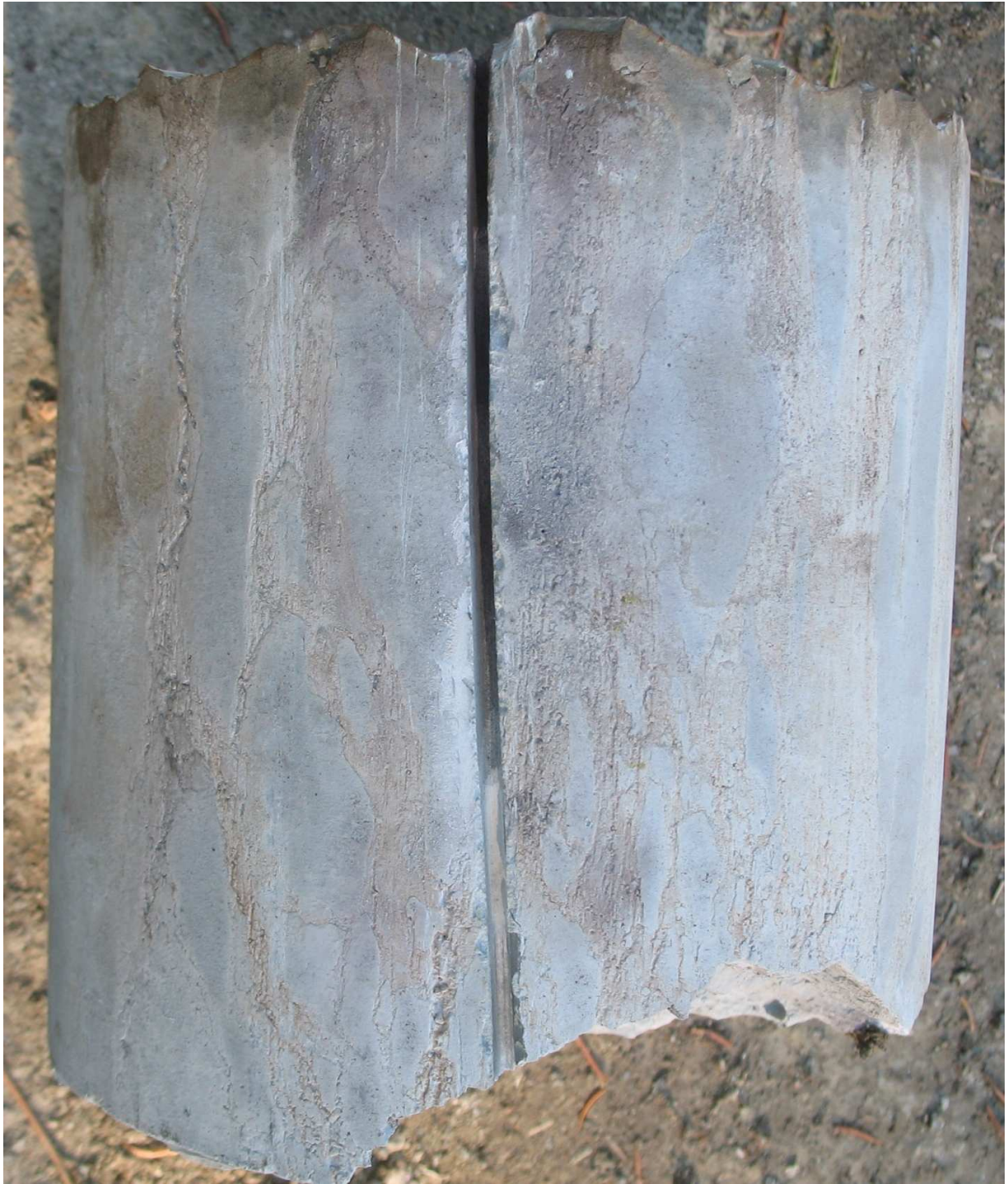
Sample 7200 Top Of Cement Plug With Water Leak Erosional Flow Paths Visible
