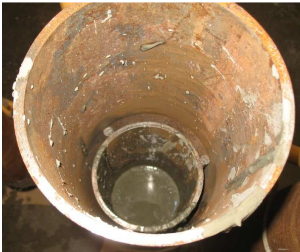
Fresh Cement Poured In Pressure Test Samples
