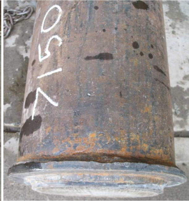
Sample 7150 With 2.0 mm Plug Movement
