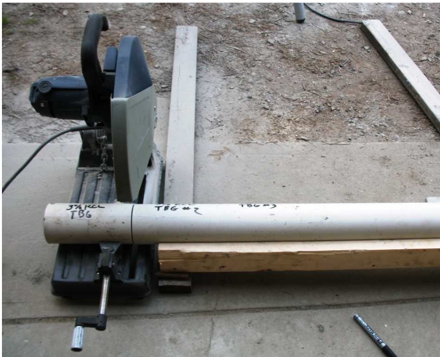
Compression Test Samples – Cutting Sample With Masonary Cut Off Wheel
