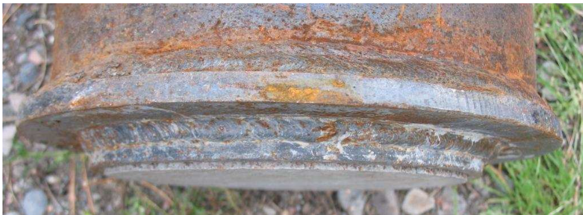
Sample 7150 With 2.0 mm Plug Movement
