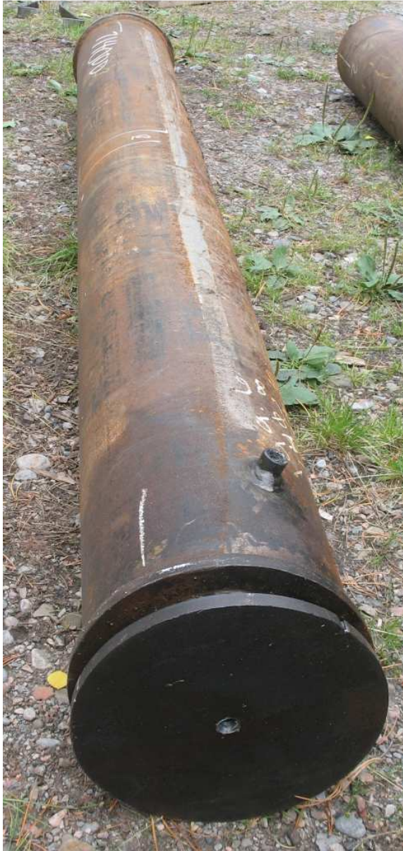
Sample 7140DD Pressure Plate End
