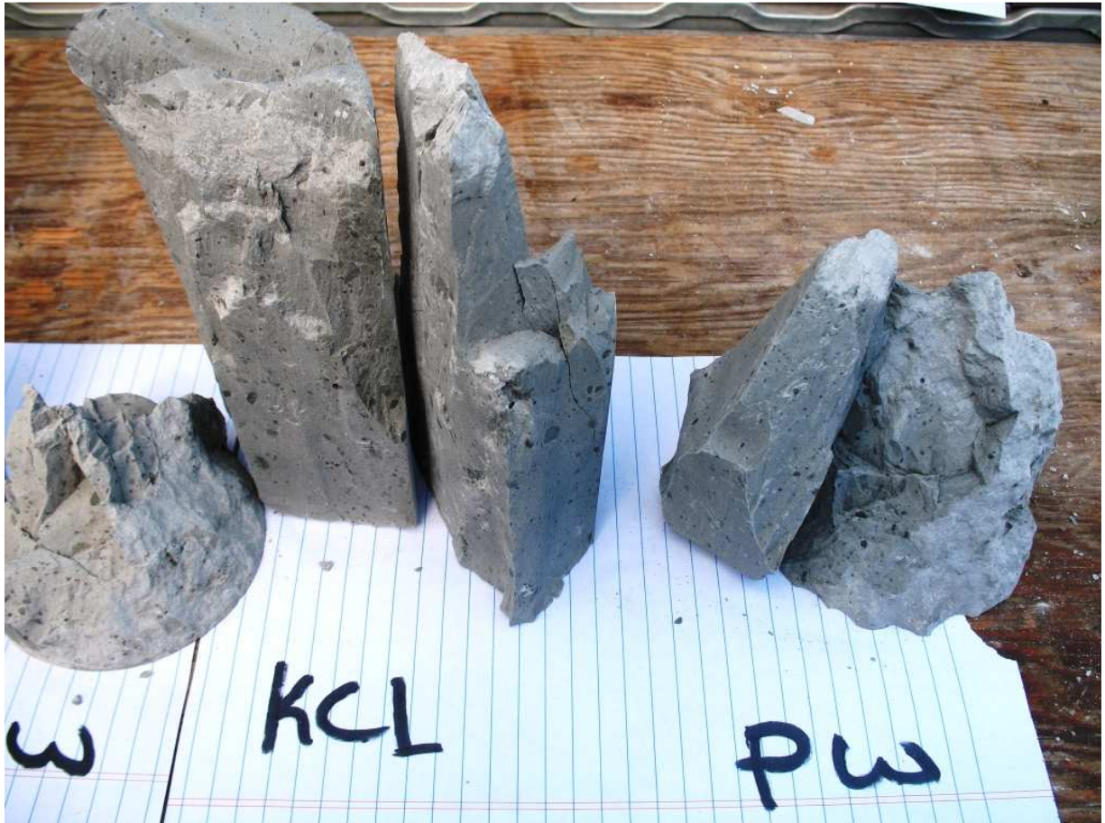
KCL and Produced Water (PW) 60 day Compression Test Samples
