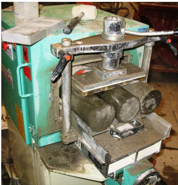
Polishing Ends On Compression Test Samples
