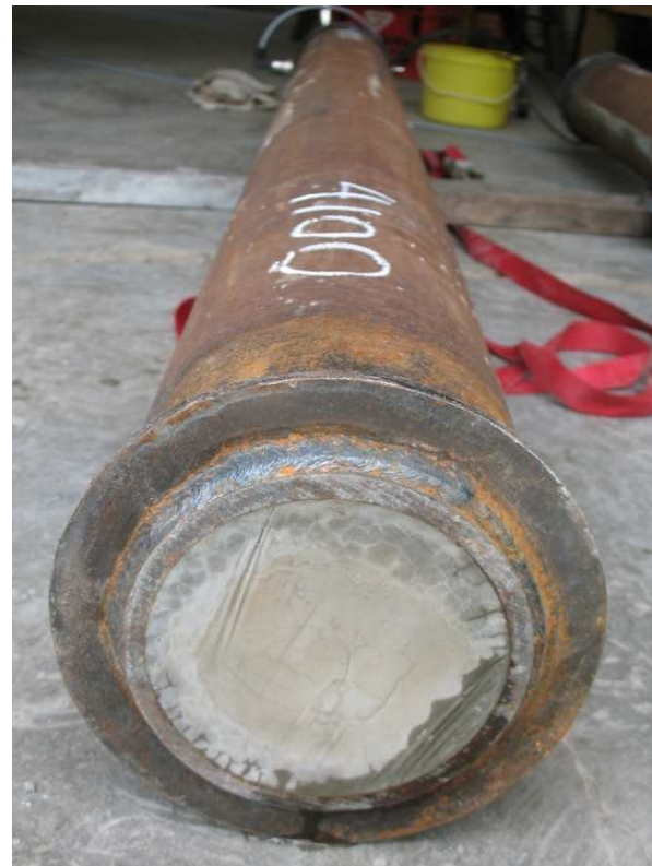
Pressure Test Apparatus Prior To Extending And Securing Hose Sample 4100 Leaking During Test
