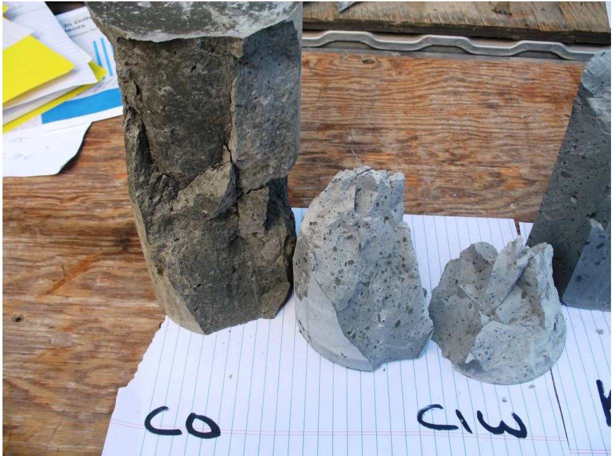
Crude Oil (CO) and Corrosion Inhibited Water (CIW) 60 day Compression Test Samples
