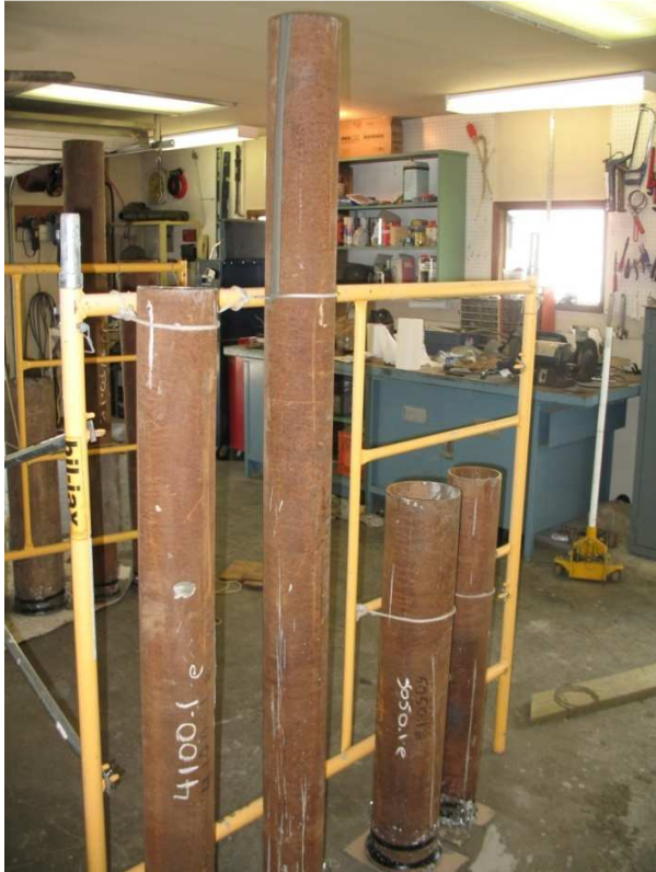
Pressure Test Samples With Cement Poured
