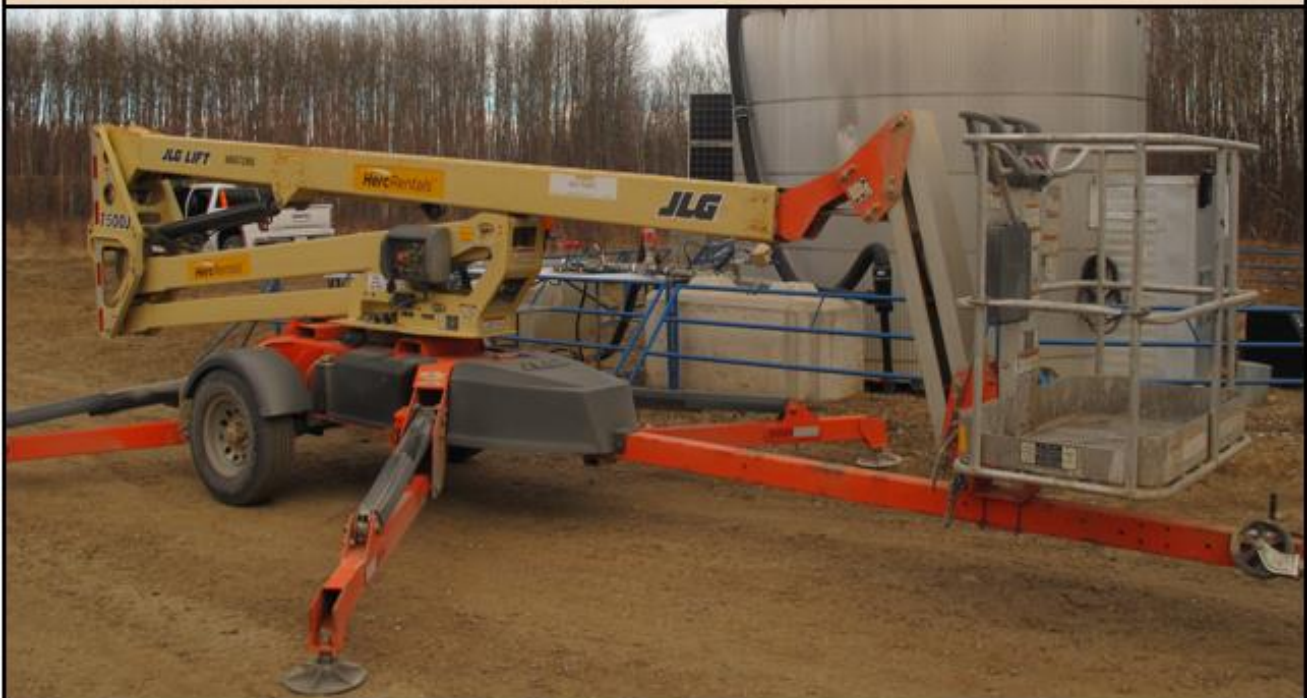
Figure B-10: 50 ft Boom Lift with Personnel Basket
