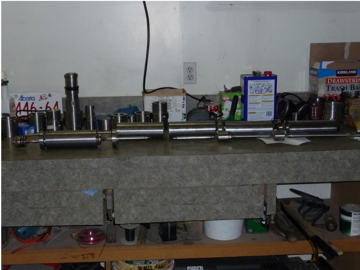
Figure 5: Bench Test of Lifteck's Gas Operated Piston Pump ©Lifteck International Inc 2012
