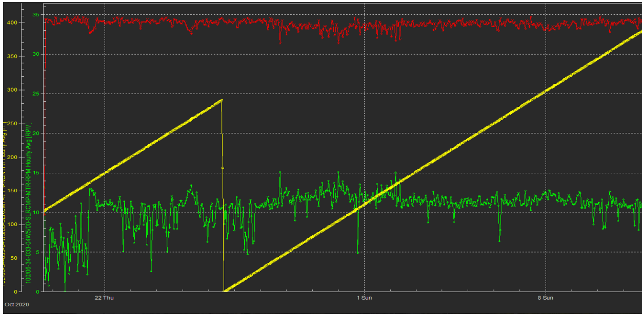
Figure 3: CROSSFIRE instrument air compressor operating trends
