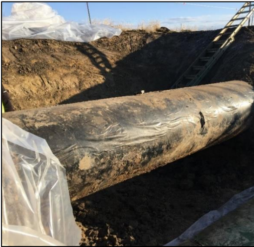
Figure 3-11: Axial wrinkling pattern along the 9 o'clock position, MP 80.4655.
