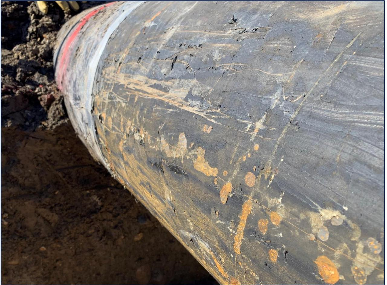
*Figure 3-5: Pitting Corrosion at 9 O'clock Position*
