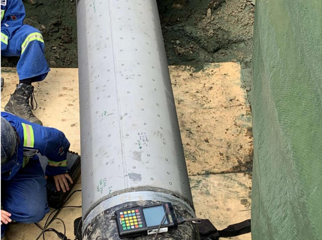
Figure T: Additional Laser Scanning of Features
