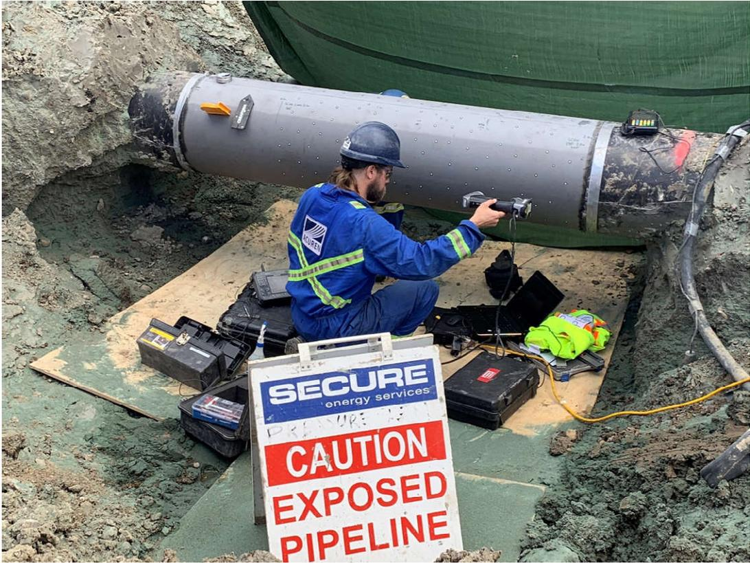
Figure S: Laser Scanning of Features
