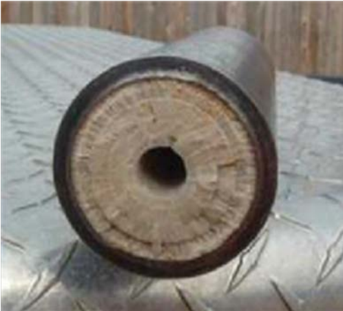
Barium sulfate in Haynesville Shale flowline after one month.
