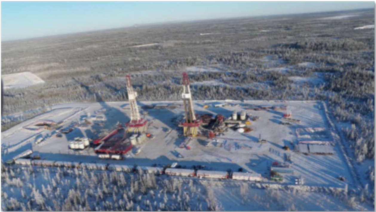
Remote locations such as the Horn River will require technological advances, such as multiple wells on a single pad to achieve economic success. (Picture Courtesy of Nexen, 2010)
