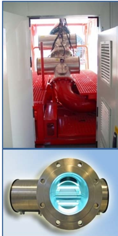
Figure 38 Tool that Uses Ultraviolet Light to Act as a Control for Bacteria
