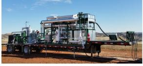
The GTUIT FCS field gas conditioning equipment takes raw gas from the wellhead and conditions it. The conditioned gas is dry, and a consistent BTU at a constant pressure with a majority of the NGLs removed. The conditioned gas can be used for field power generation, compressed natural gas, liquefied natural gas, and gas-to-liquid feed stock.
