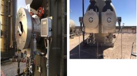
The Rush Burner's patented burner system achieves 99.99% total hydrocarbon destruction, and combustion efficiencies of 80% at pressures as low as two ounces. The Rush Burners can either use onsite power or the available solar package option. Incorporating safe and reliable ignition/flame sensing in the design creates a unique flame profile that increases heat transfer, inhibits flame lift off, and eliminates fire tube impingement. All Rush Burners come complete with:
