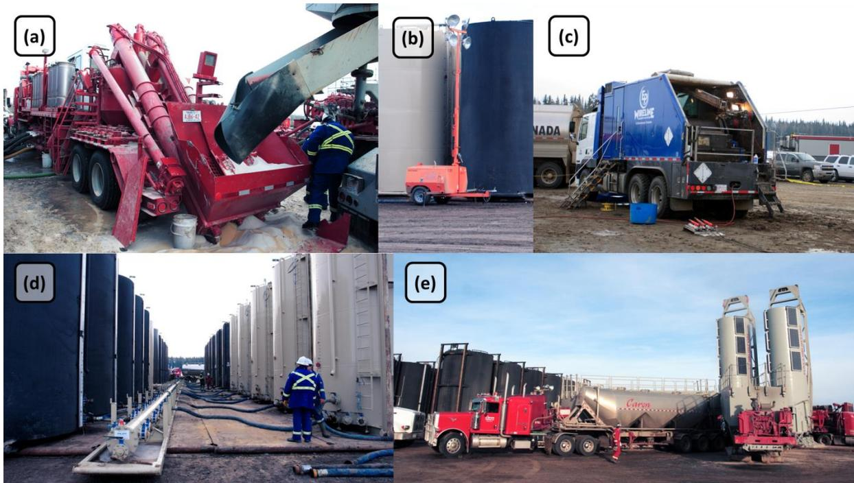
**Figure 4.5: (a) Blender truck receiving sand, (b) Diesel powered light stand, (c) Wireline truck, (d) Heated water tanks, (e) Sand conveyor**
