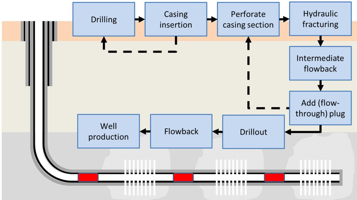
**Figure 2.3: Schematic well-completion diagram and depiction of a fractured horizontal well with plugs before drillout**
