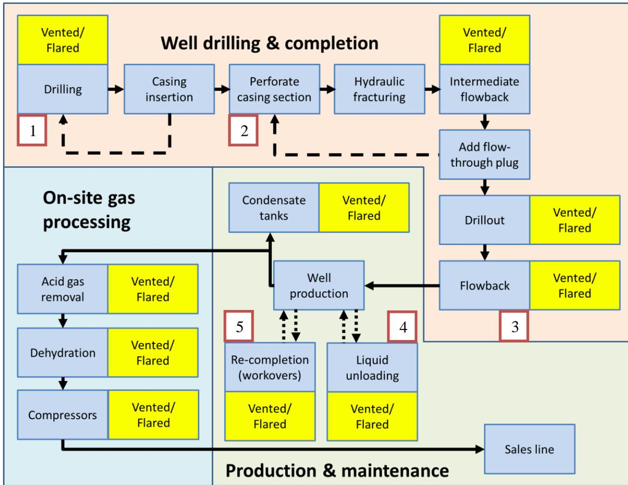
**Figure 2.1: Schematic of key processes involved in well drilling & completion; production & maintenance; and on-site processing of hydraulic fractured unconventional gas**
