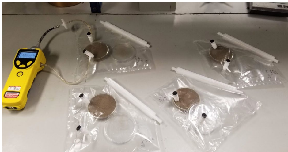
Figure 5. Photoionization detector attached to Tedlar® bag containing spiked soil. 1 of 4 replicates containing PHC F2-spiked soil at approximately 10,000 mg/kg.
