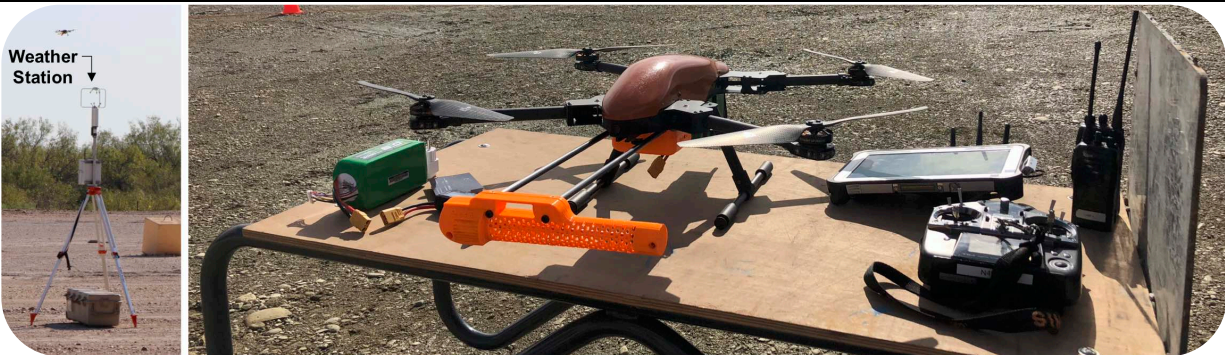
Figure 1. SeekOps field kit consisting of Weather Station, Drone and Associated HW.
