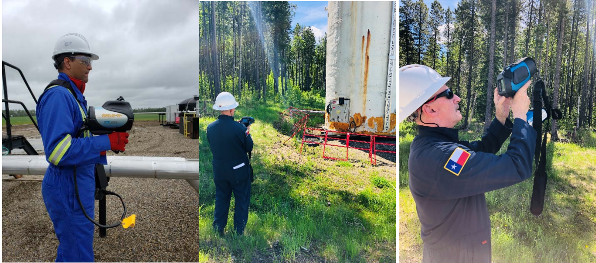
RMLD-IS (left); RMLD-CS (right two): The RMLD-IS and CS are high sensitivity open path lasers capable of detecting small methane plumes from a distance.
