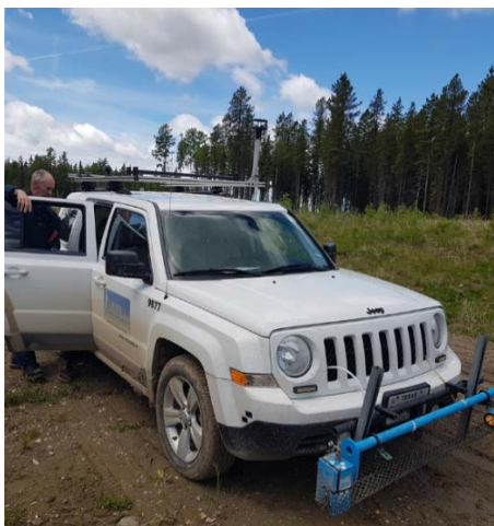
OMD Mobile survey: The OMD is an open path methane specific sensor capable of detection of small plumes. It is specifically designed to survey under harsh conditions.
