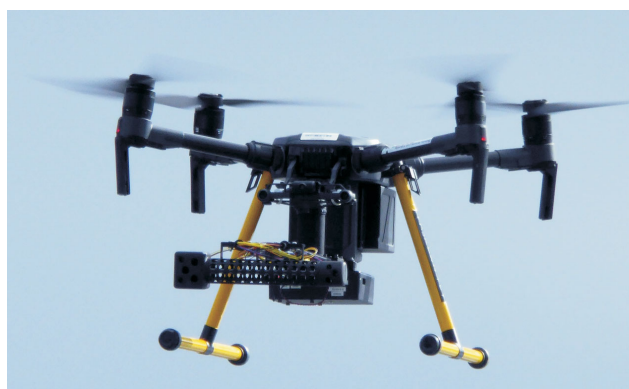
Figure 1. The GHGMapper™ system with open path laser spectrometer/small unmanned aerial vehicle (OPLS/sUAV) platform.
