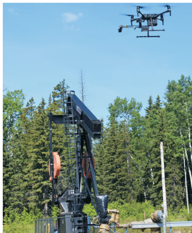
Figure 2. The GHGMapper™ system (open path laser spectrometer/small unmanned aerial vehicle platform) surveying at an Alberta Methane Field Challenge facility, June 2019.
