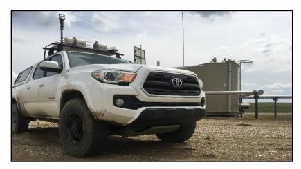
Left: The University of Calgary Portable Methane Leak Observatory (PoMELO) conducting emissions surveys. The system is mounted on the roof of conventional field truck and is completely computerized.
