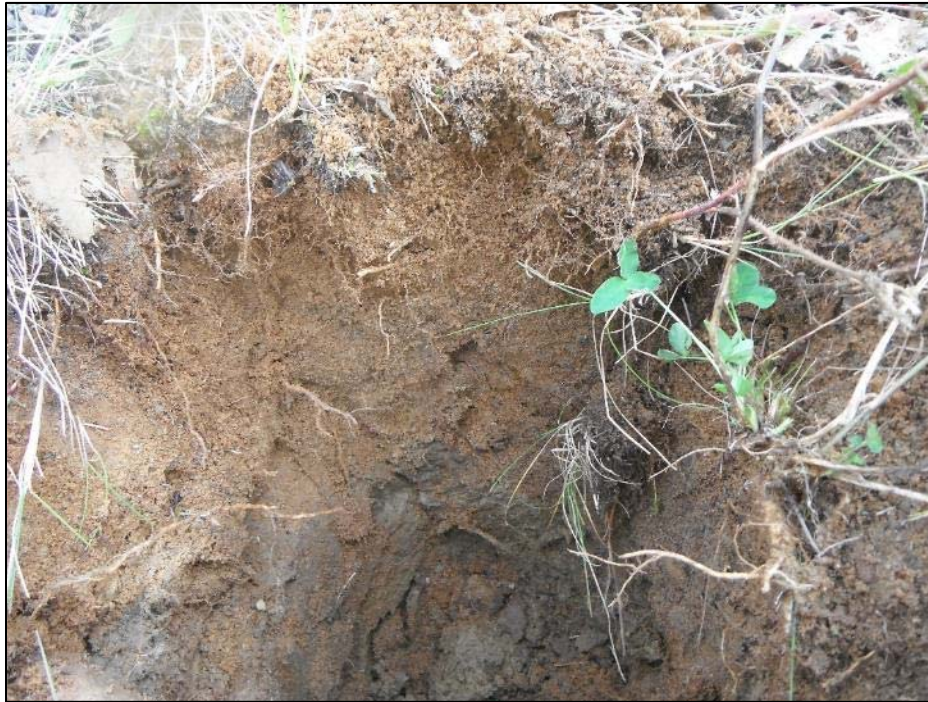
Photo 11. Soil profile with no topsoil on the wellsite
