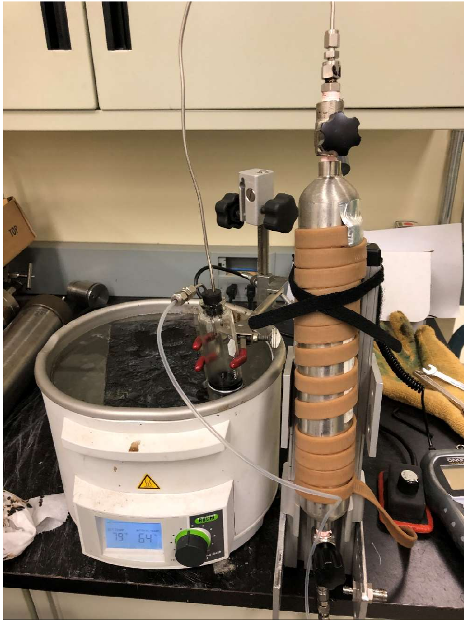
Fig. 23 — Sample cannister and heated bath
