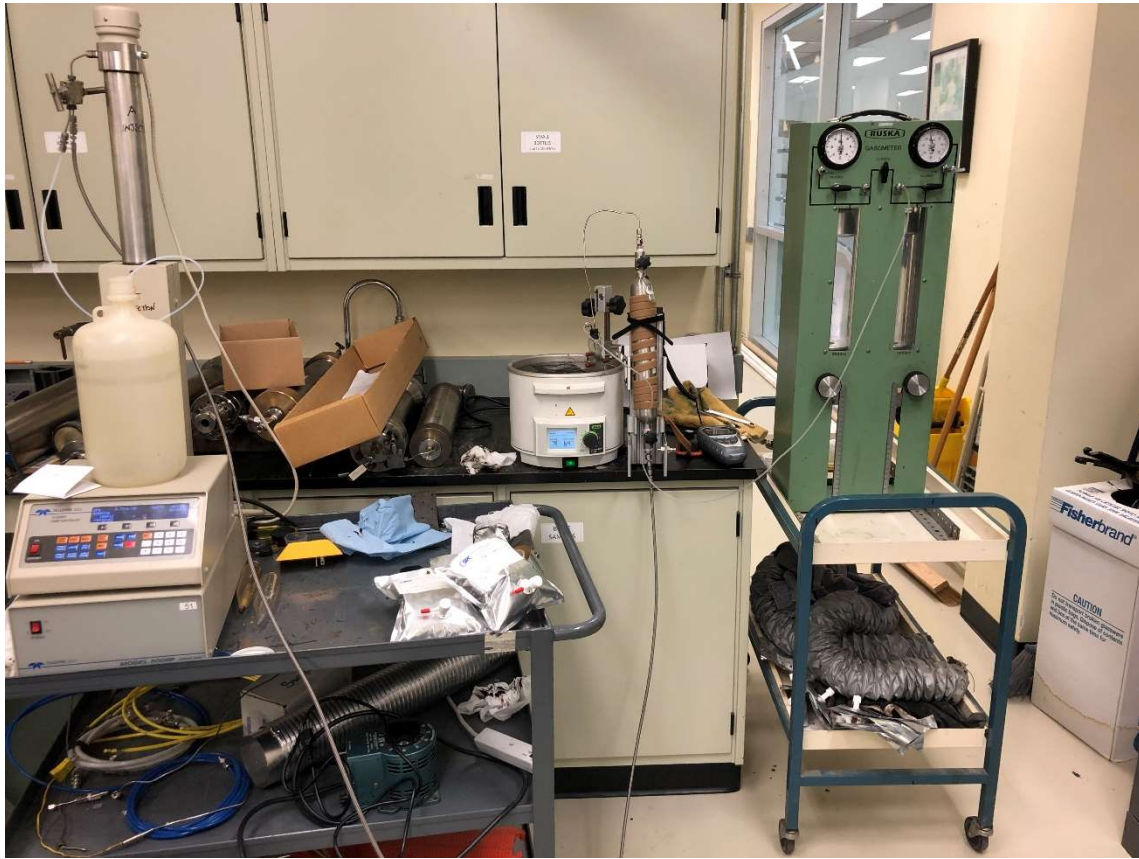
Fig. 22 — Total set up for GIS samples. On the left is the syringe pump, middle is the heated bath and sample container, and gas meter on the right
