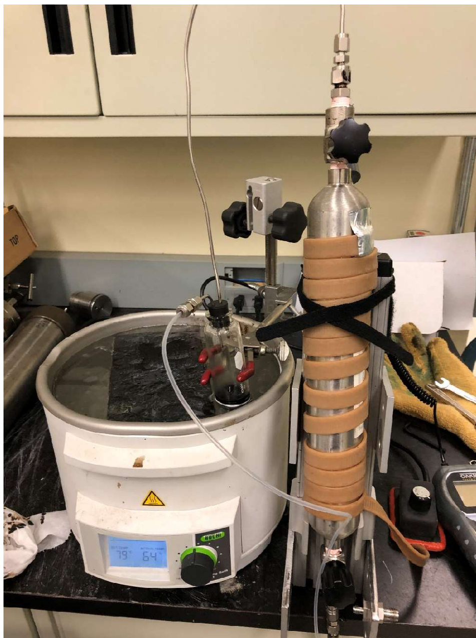
Fig. 23 — Sample cannister and heated bath
