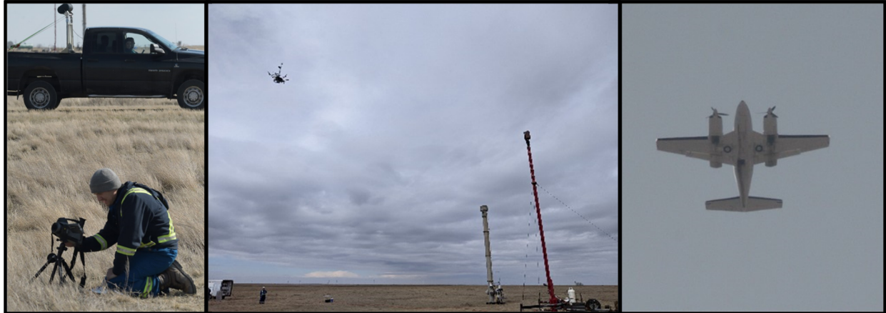
Figure 4: Participants of the first field campaign included two QOGI systems, truck- and drone-mounted TDLAS, and airborne SWIR hyperspectral imaging.
