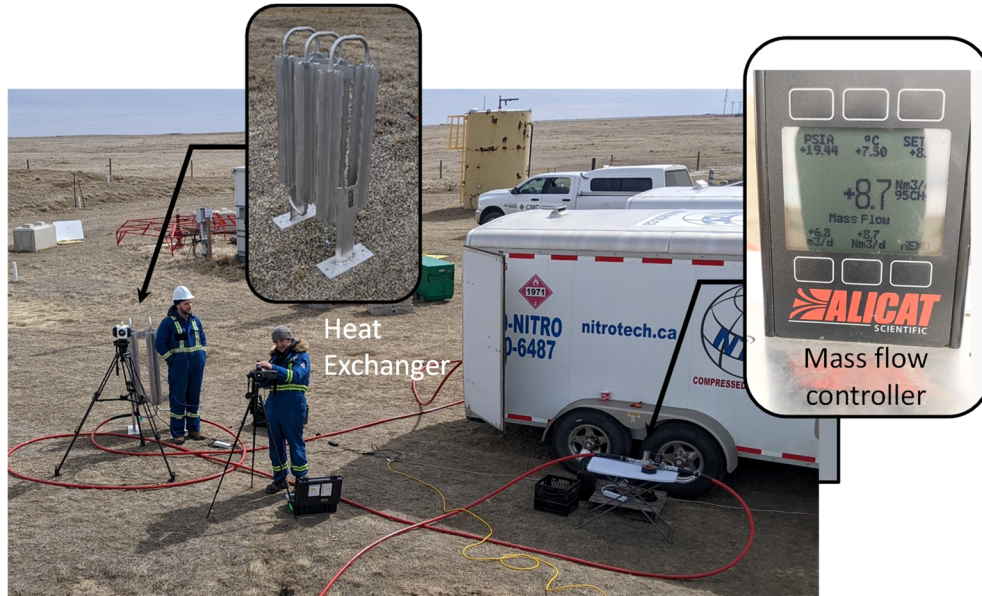
Figure 5: Methane was released from compressed cylinders in a trailer, through a heat exchanger, and then into a mass flow meter, before exiting a nozzle, stack, or the unlit flare.
