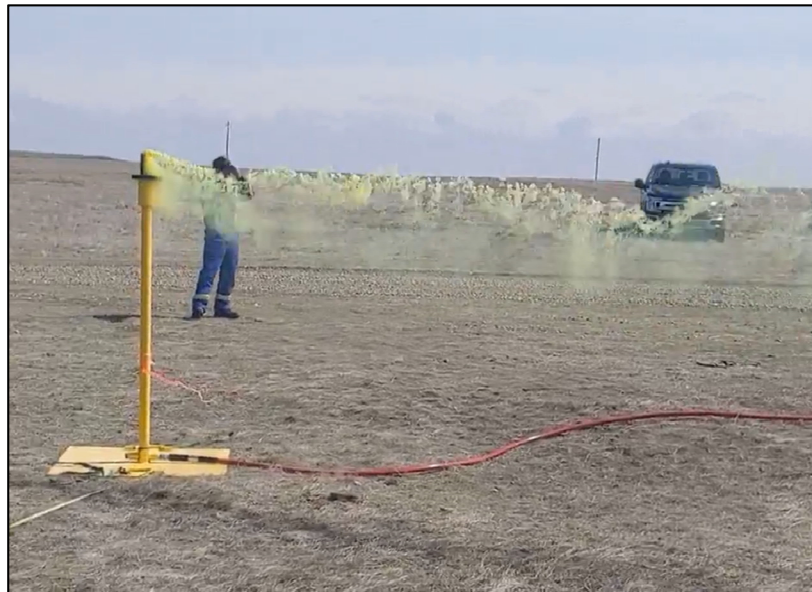
Figure 17: Example smoke release test. The dispersion of smoke suggested that the ambient wind was pushing the methane towards the ground.
