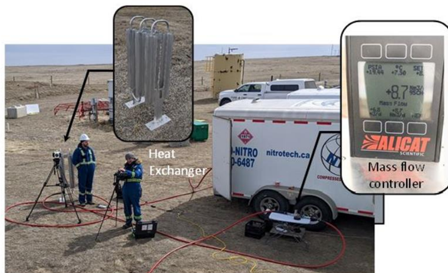
Figure 6: Controlled release setup
