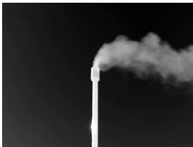
Figure 30: QL320 measurement #24, sample image showing the raw capture of the release without any overlays. The plume is relatively dense throughout which reduces the contrast within the plume and may make velocimetry less accurate.
