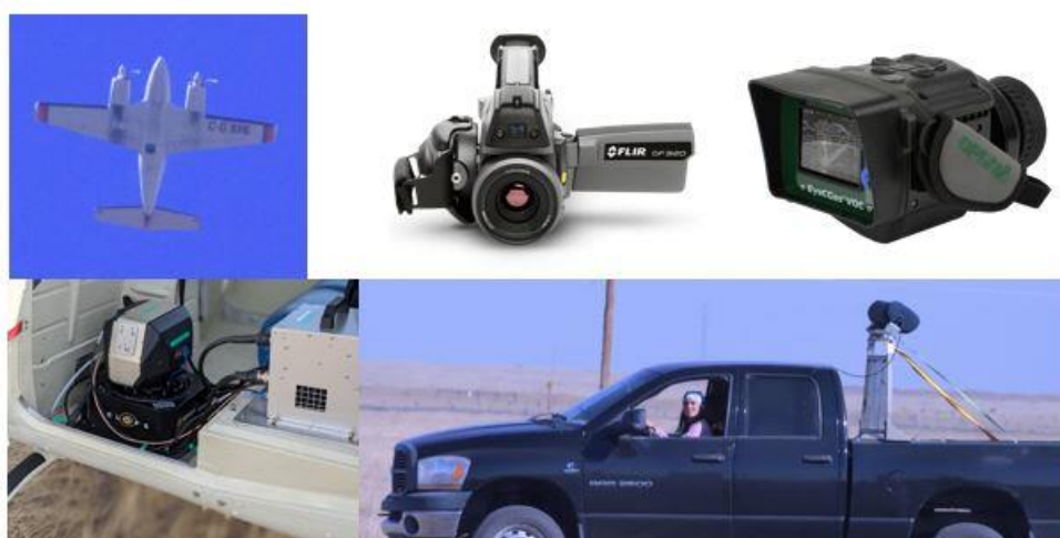
Figure 7: Participating technologies in September 2022 field trials. From left to right, top to bottom: Airborne NIR HS Imaging; FLIR GF320 QOGI; OpGal QOGI; Airborne LWIR HS Imaging; Truck-based TDLAS
