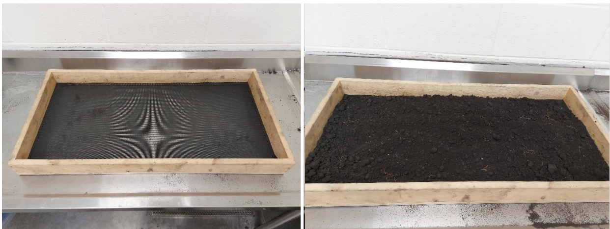
Figure 11. Frames used for root sieving. The photo on the left shows the frame without soil, and the photo on the right shows a frame with soil prior to sieving.
