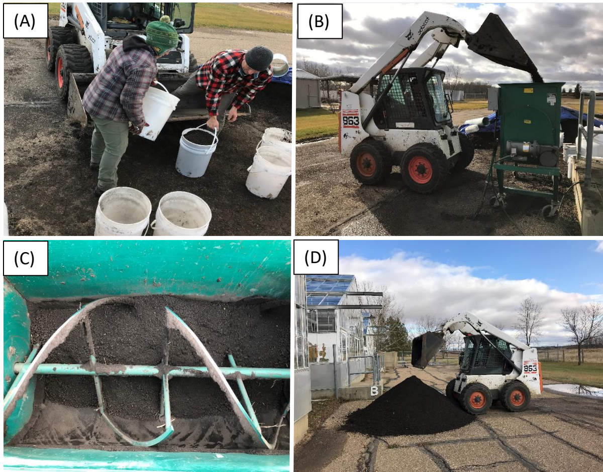
Figure 4. Spiking soil with NaCl.
