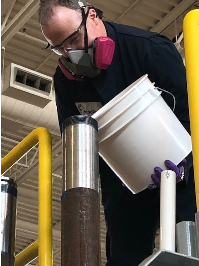
Figure 4: Placing Resin Into Casing And The Casing Stub With Aluminum Centralizer
