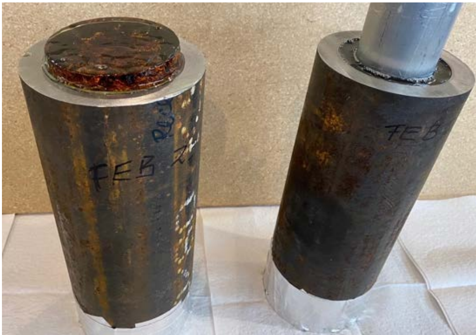
Figure 11: Resin Curing / Extruding from Casing Stub and Casing Stub With Centralizer
