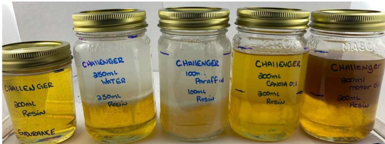
Figure 7: Resin Curing In Various Fluids In A Paraffin Lined Container And An Empty Container
