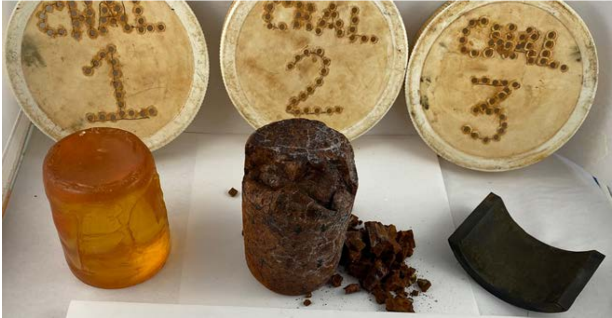
Figure 20: Resin, Class G Cement & J55 Steel Samples After 194 Days Of Endurance Testing
