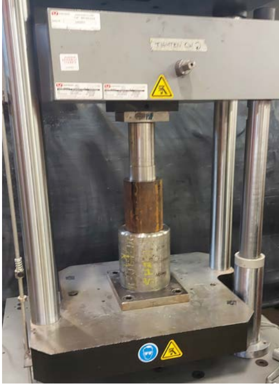
Figure 14: Intron Satec 600 DX Load Frame With a Casing Stub in Position
