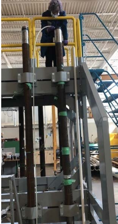
Figure 3: Casing Preparation And placing Wiper Plug Inserts
