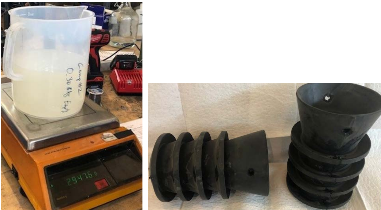
Figure 2: Measuring Resin Components And Wiper Plug Insert
