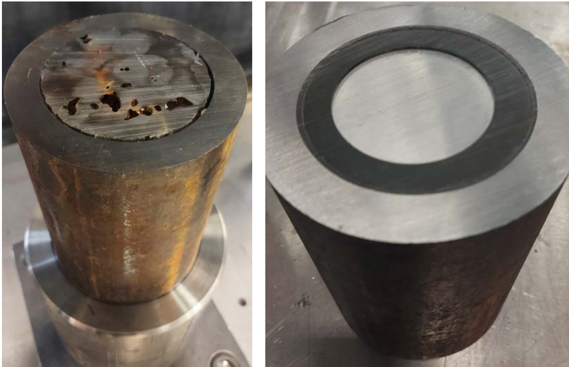
Figure 13: Casing Stubs With Resin Prepared For Shear-Adhesion Testing
