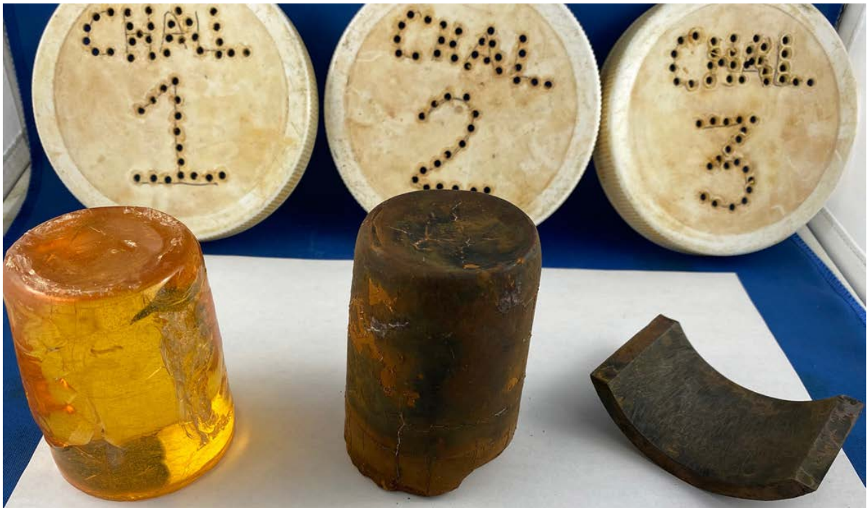
Figure 19: Resin, Class G Cement & J55 Steel Samples At 90 Days Of Endurance Testing
