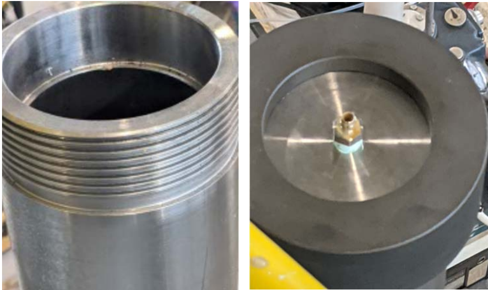
Figure 1: Machined End Connections On Casing
