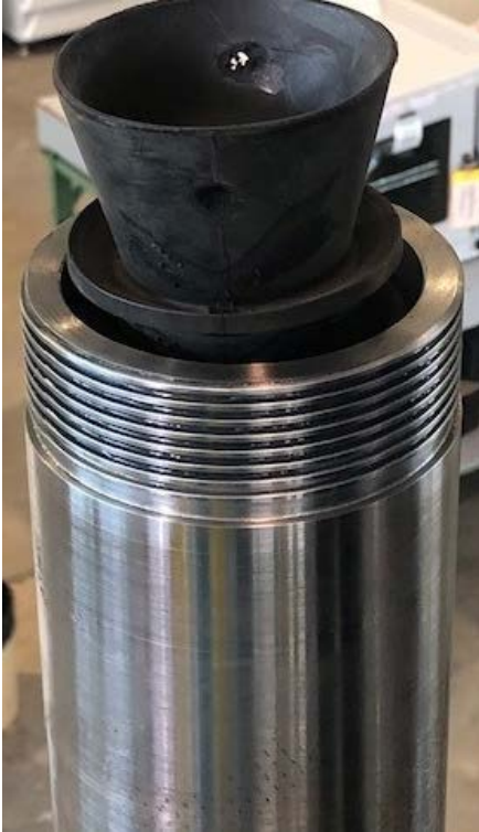
Figure 3: Casing Preparation And placing Wiper Plug Inserts
