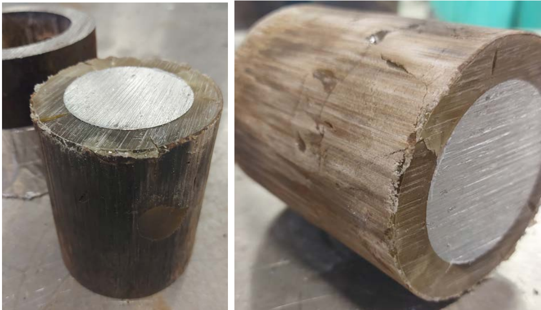
Figure 15: Resin With Centralizer Pushed Out Of Short Casing Stub
