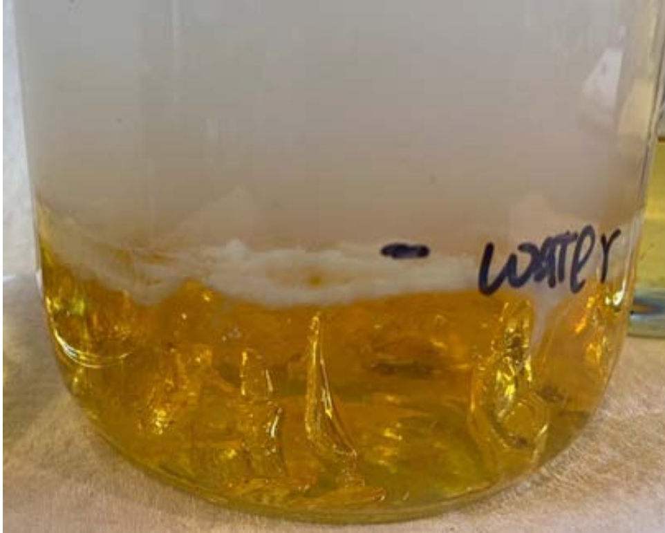
Figure 10: Resin Cured In Water With Voids And Some Top Foam
