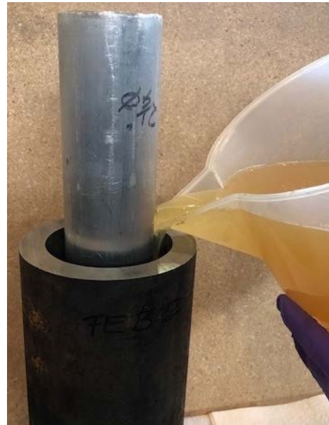
Figure 4: Placing Resin Into Casing And The Casing Stub With Aluminum Centralizer
