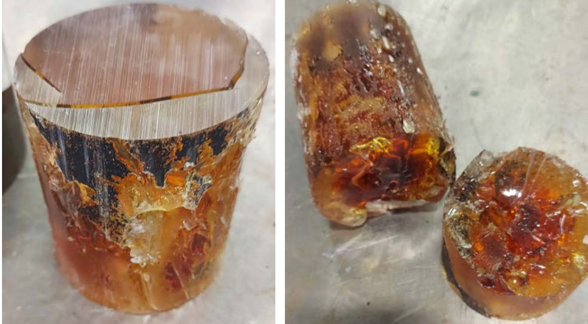
Figure 16: Resin With No Centralizer Pushed Out Of Casing Stub
