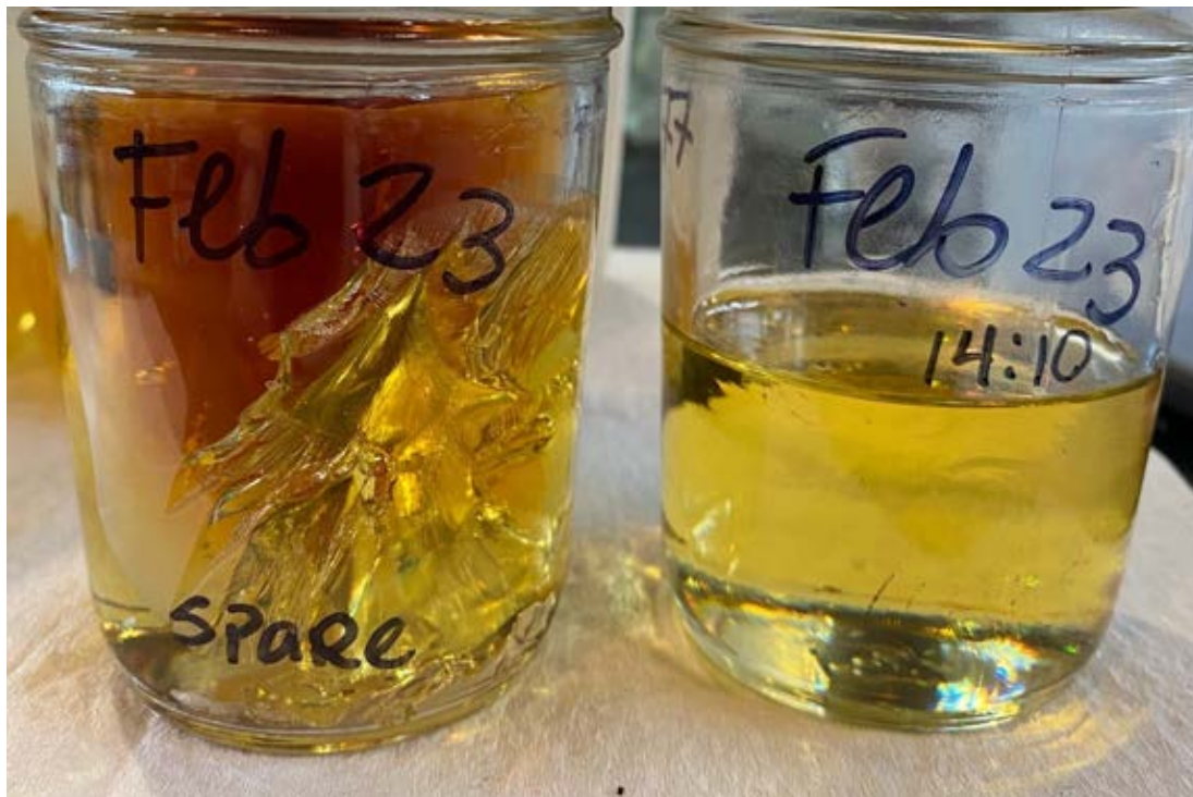
Figure 9: Resin Samples With And Without Voids
