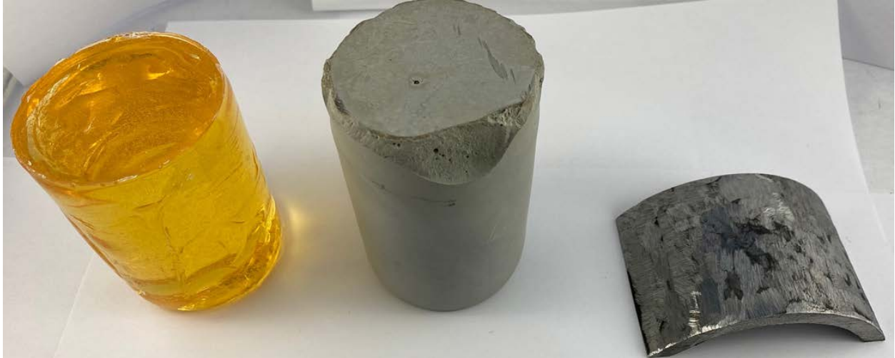
Figure 18: Resin, Class G Cement & J55 Steel Samples Before Endurance Testing
