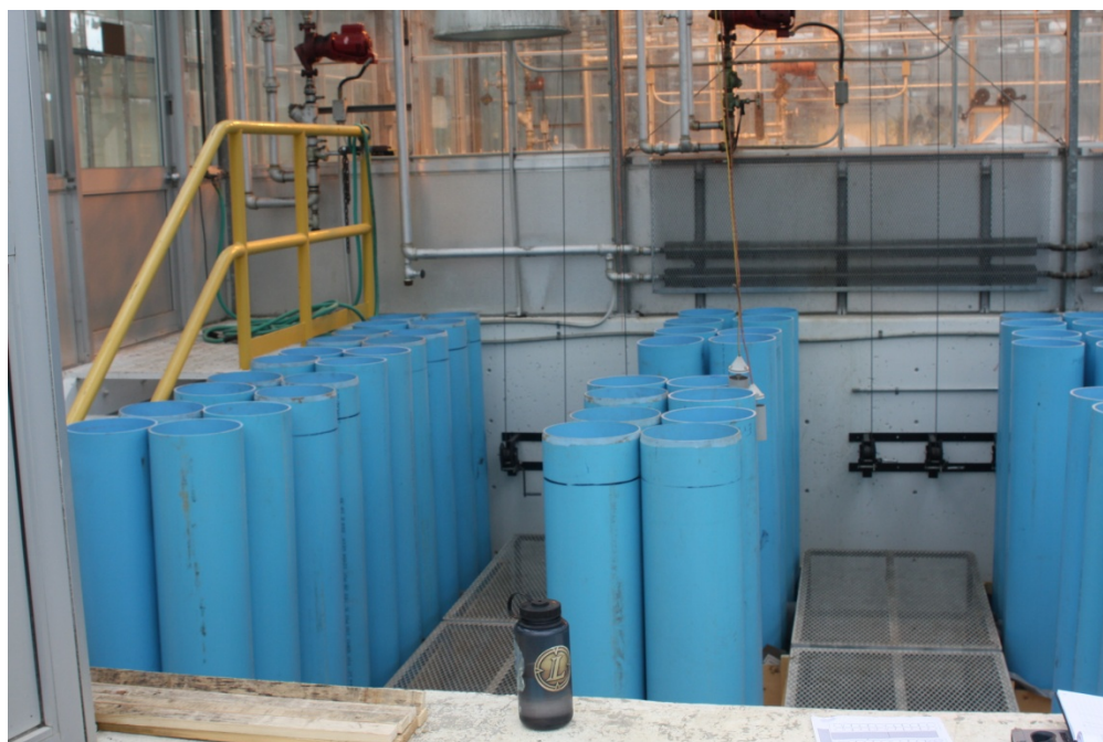
Plate 5. Soil columns installed in watering boxes in the sunken greenhouse in Vegreville.
