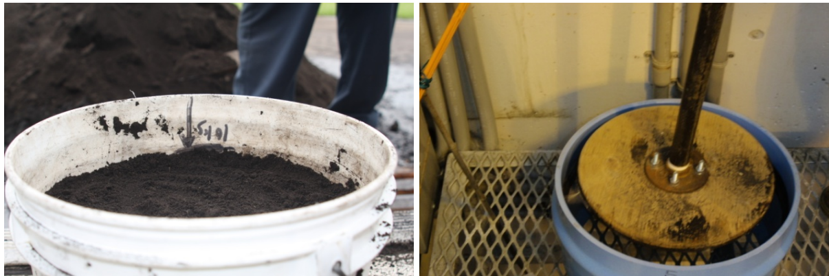
Plate 8. Calibrated bucket and tamping tool used to achieve targeted bulk density.
