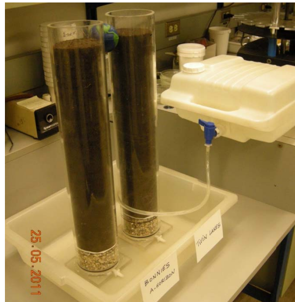
Plate 11. Lab study to evaluate the effect of bottom watering boxes and capillary rise.
