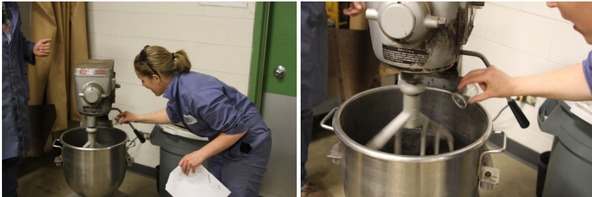
Plate 6. Adding predetermined amount of F2/F3 PHC to 10 kg soil in small mixer.
