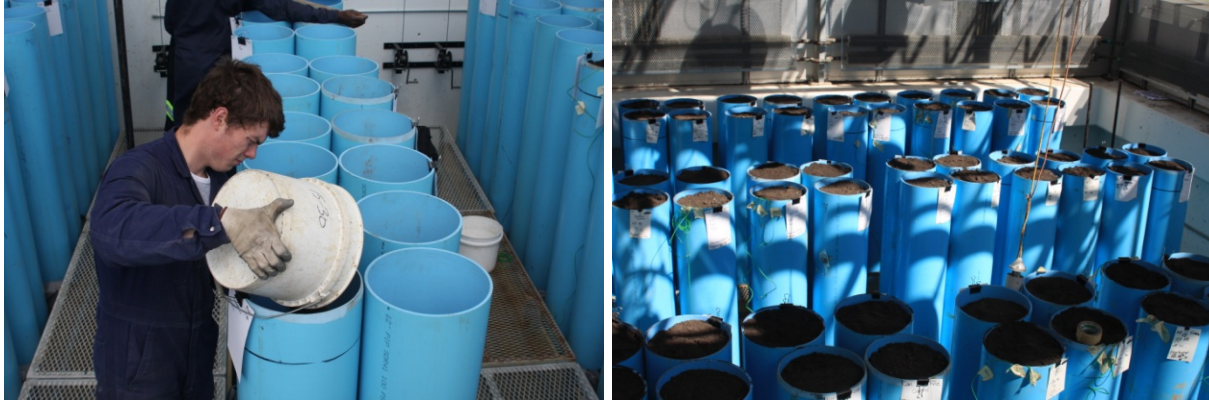
Plate 9. Adding soil to columns to achieve the required depth.
