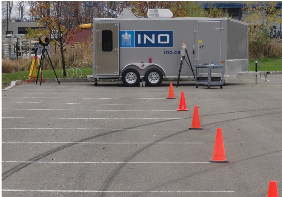
Figure 7. Site installation of INO mobile laboratory (folding mirror in front of open doors).
