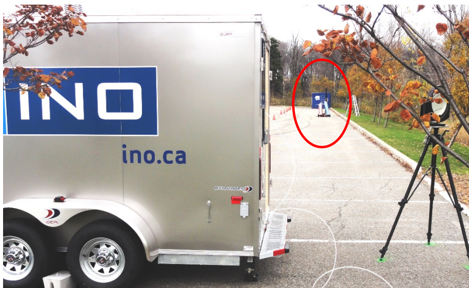
Figure 8. Mock-up stack with gas bottles at the end of the stand-off path.
