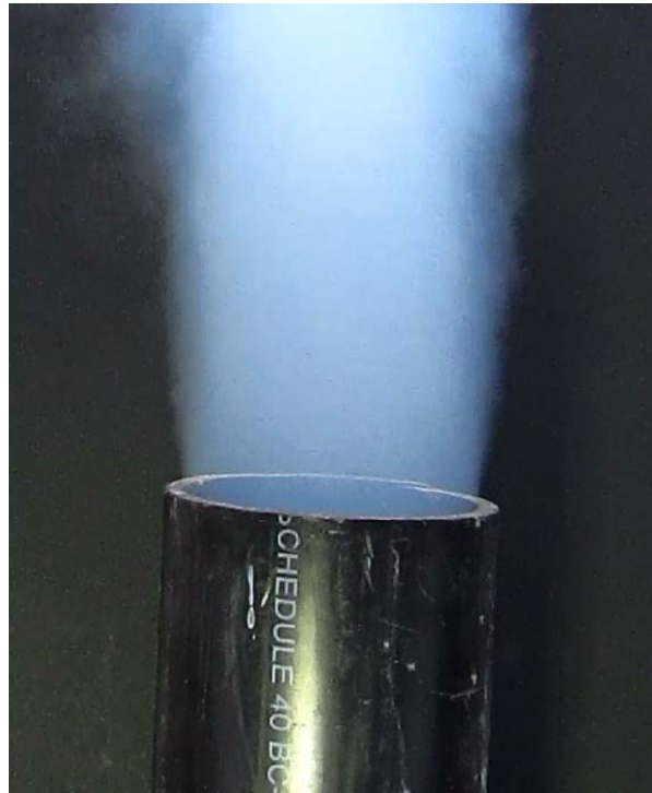
Figure 5. Fumes outputted from the mock-up stack at ~5 m/s.
