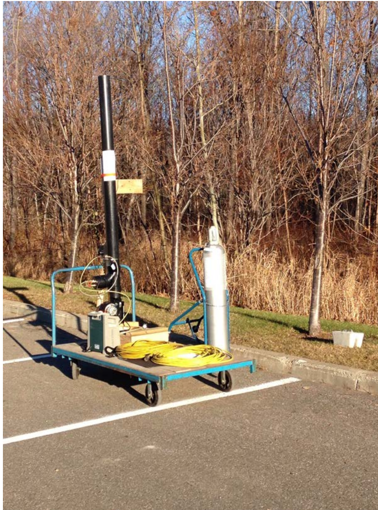
Figure 4. Photo of the ambient temperature mock-up exhaust stack and gas cylinders.
