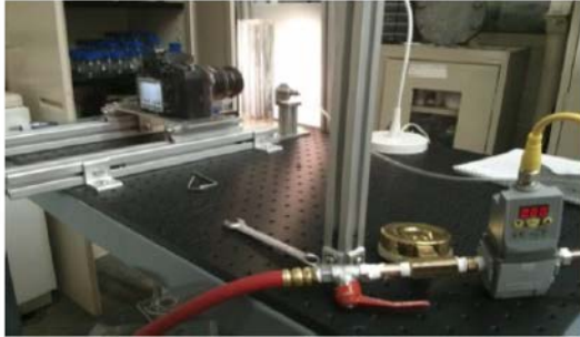
i. Air is injected into carbopol. Injection pressure is controlled with pressure regulator.
