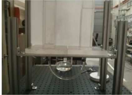
ii. Controlling injection pressure with manometer.
