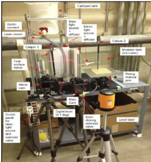
iii. Invasion pressure is controlled by making difference in fluids level. The height difference is applied with lifting up the column of water by a scissor jack under the water tank.
