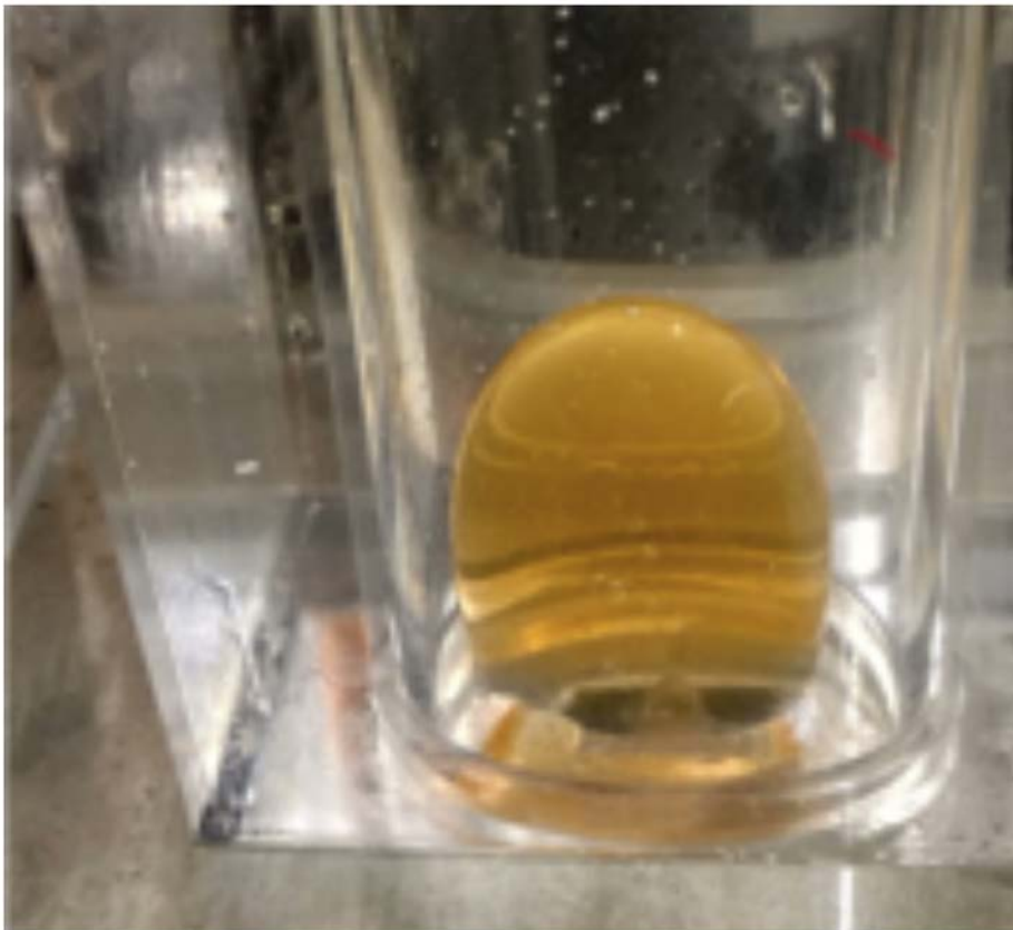
Figure 28: Invasion of R550 into a density matched (0.15% wt) Carbopol solution of height H=10 radii
