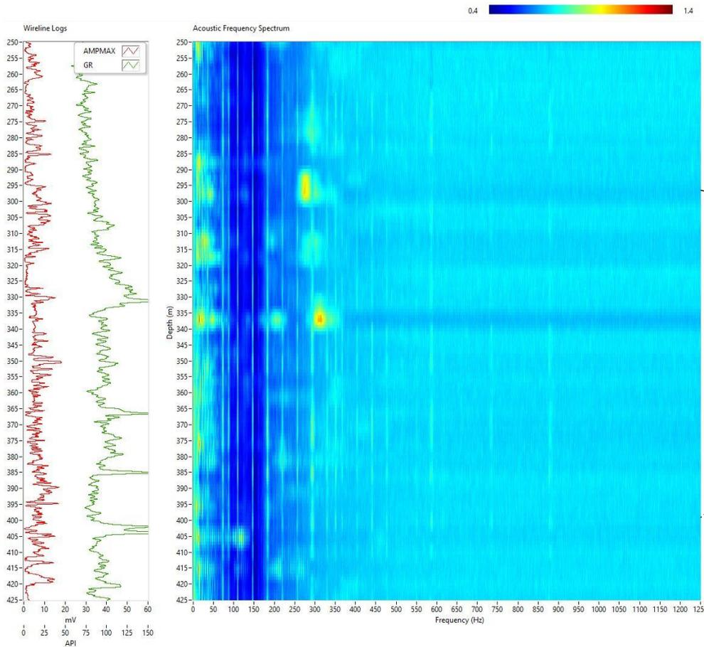
A zoomed in view of the acoustic frequency spectrum shows the most intense part of the signals are positioned at 297 m, 337 m, and 406 m. A greater confidence is placed on the two shallower signals (297 m and 337 m) as there is a more intense response. The signals near 0 Hz and the vertical lines present throughout the spectrum are artefacts from the processing.
