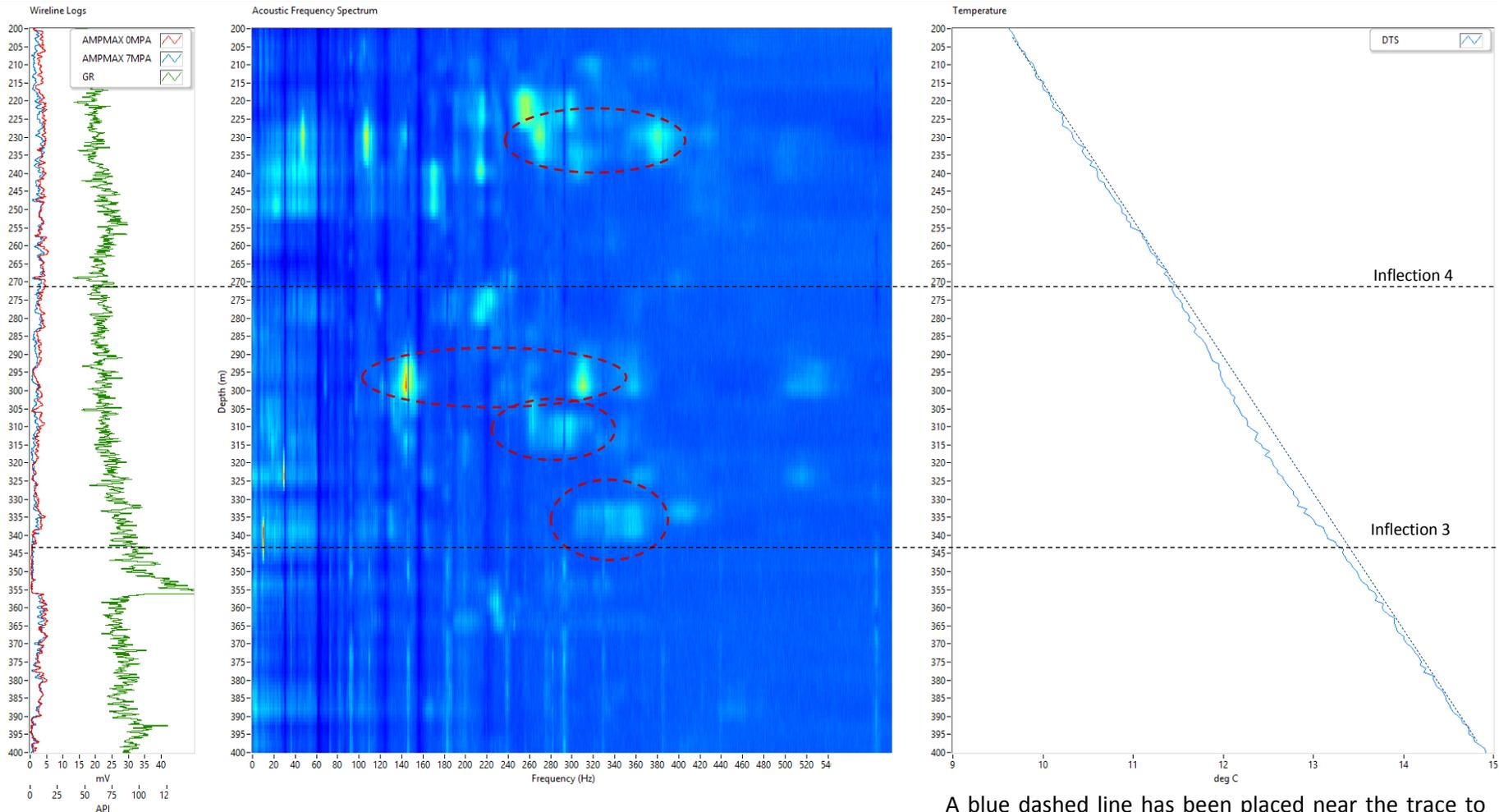
A zoomed in view of the acoustic frequency spectrum shows the most intense part of the signals are positioned at 229 m, 299 m, 310m, and 336m. A greater confidence is placed on the two shallower signals (229 m and 299 m) as there is a more intense response at distinct frequencies. The signals near 0 Hz and the vertical lines present throughout the spectrum are artefacts from the processing.
