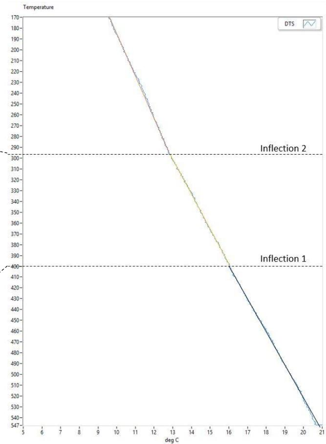
Colored straight lines were placed over the DTS trace to identify the inflections. Where the color changes is where there was an inflection point. Inflection 2 at 297 m was a stronger response than Inflection 1 at 400m. Note: the temperature plot is not on the same depth scale as the acoustic frequency spectrum so the dashed lines were extended over to the acoustic
