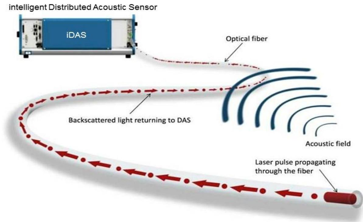
*Figure 1 Principle of operation of the intelligent Distributed Acoustic Sensor (iDAS)*
