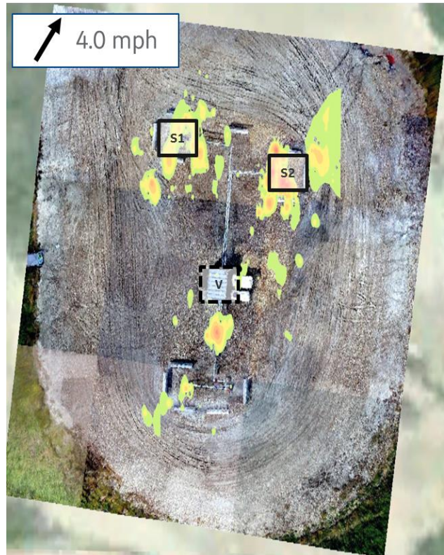
Figure 22. Multiple Leak Source Locations
