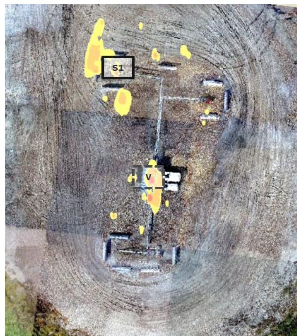
Figure 15. Detected Plumes at Wellsite
