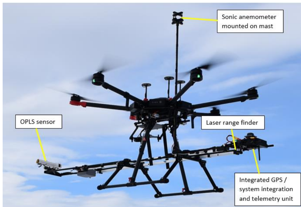
Figure 6: OPLS and redesigned mount attached to M600 platform, as used in the March field campaign.
