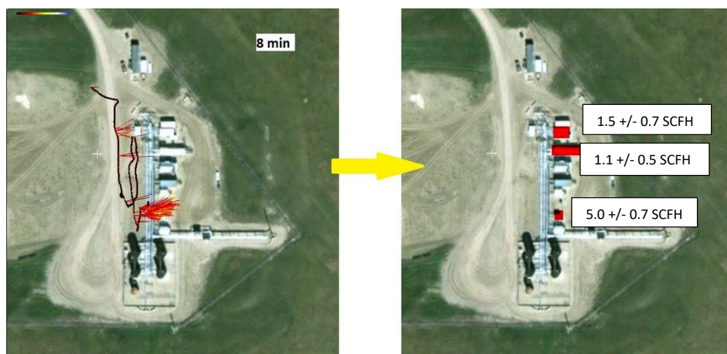
Figure 19: Leak localization from Flight 5 data.
