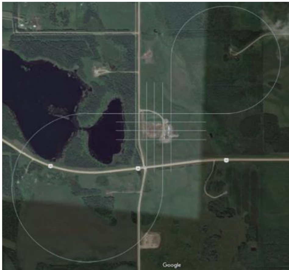
Figure 9. Example facility scan mission plan for Site 12-31. Flight path lines indicated in grey are offset such that successive passes result in coverage of the entire facility.
