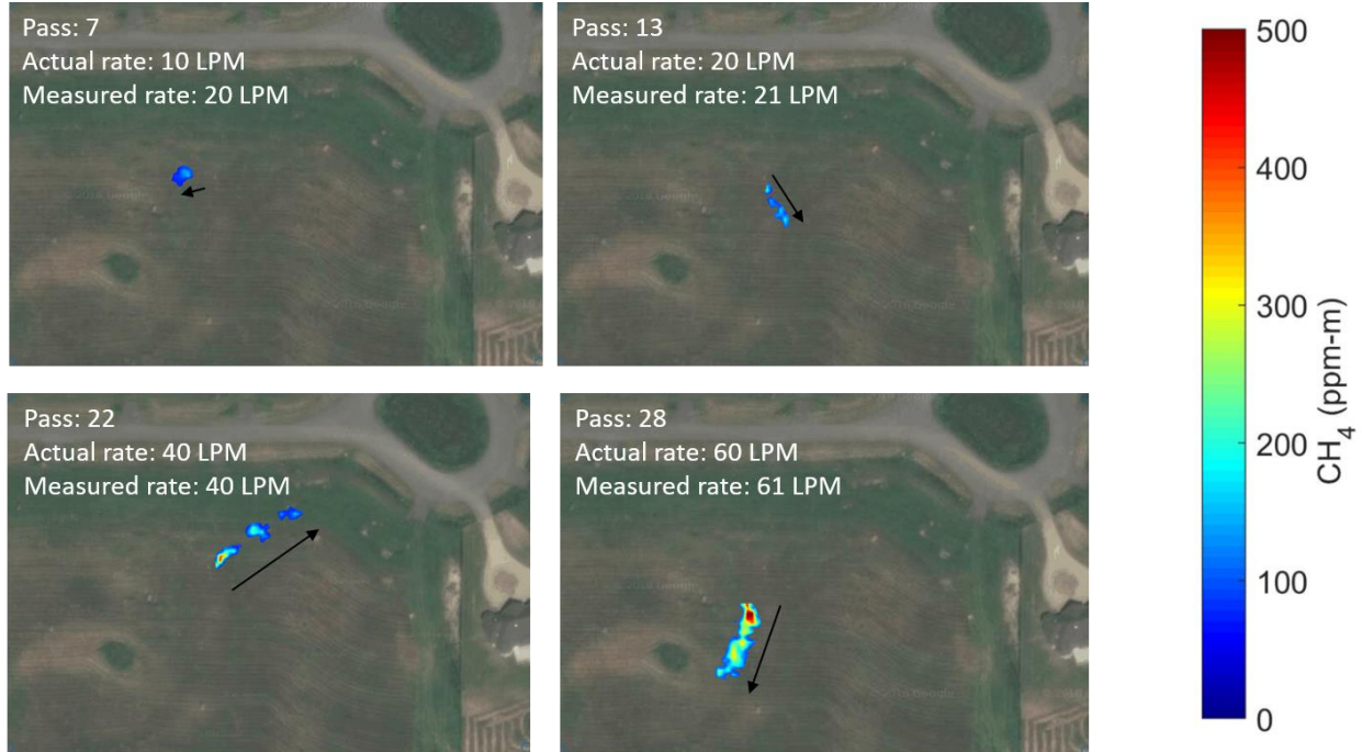
Figure 11. Controlled release plume images for the four emission rates. The arrows next to the plume indicate the wind direction and velocity at the time each image was acquired.
