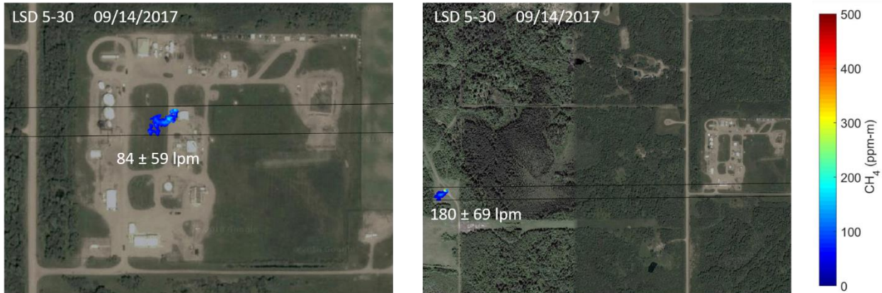
Figure 17. LSD 5-30 facility scan flight passes acquired on 9/14/2017. The black lines indicate the measurement swath for the displayed flight passes, and flux estimates are shown next to each detected plume. The right image shows a leak that was detected on a smaller adjacent facility adjacent during the LSD 5-30 scan.
