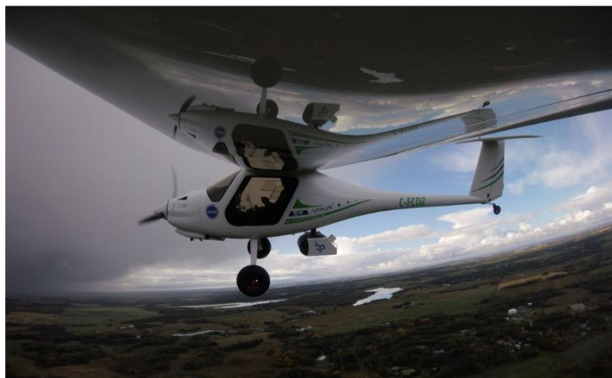
Figure 2. Left: GML mounted on the Pipistrel Virus SW1 during a flight test near Edmonton, AB. Right: Performance specifications of the prototype GML used for the testing described herein. Production GML sensors will have improved performance in nearly all areas, see Section 7 for details.
