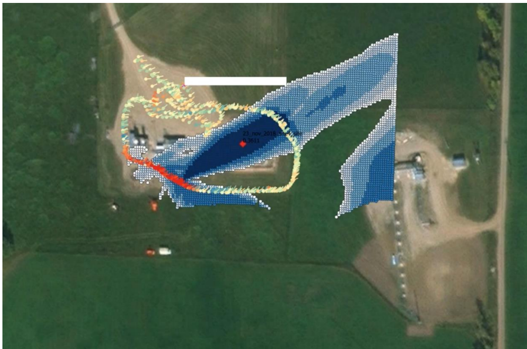
Fig. 9: Map showing methane concentration and wind direction during a survey of a facility in November 2018. Wind direction was from the northeast. The name and location of the facility has been redacted. The colored points with lines are the methane concentrations (red denotes higher concentration) and wind directions. The colored area shows the emissions source probability map, with the candidate source denoted by the red diamond. In this case the source identified by our localization algorithm corresponded to a tank.
