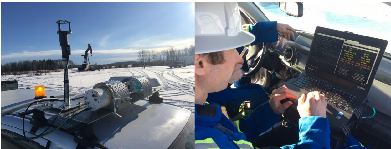
Fig. 1: The PoMELO hardware (left) and PoMELO Live software (right). The vertical mast is the wind sensor. The methane sensor is covered by two metal shields. The GNSS is on the far side. Power is supplied from inside the vehicle.
