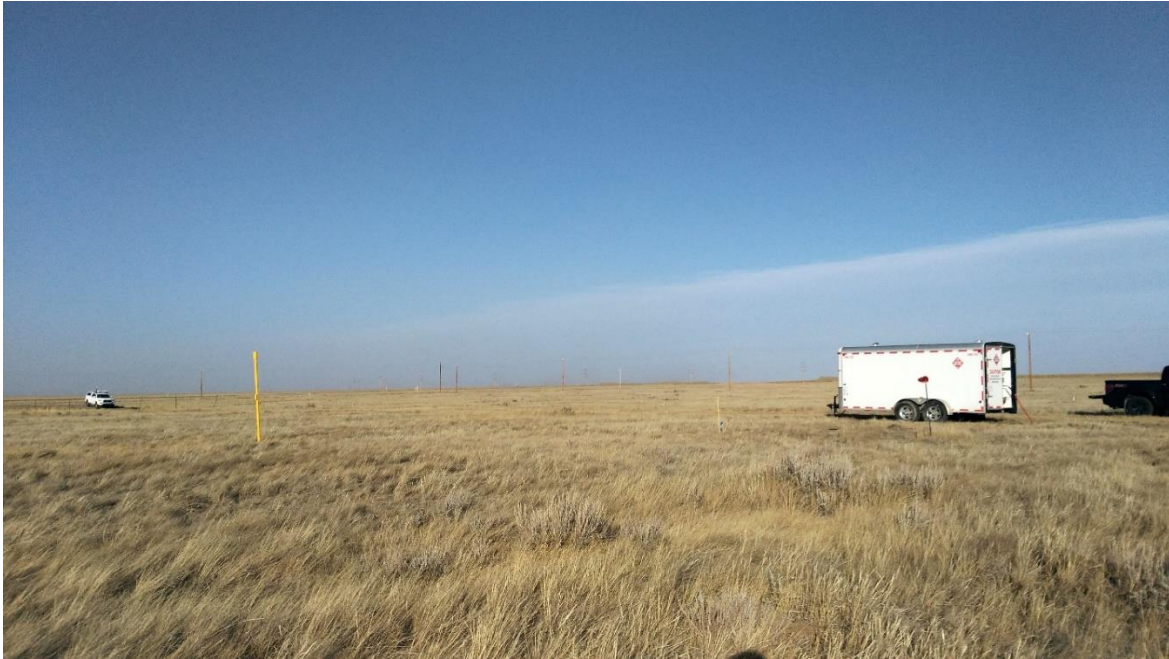
Fig. 5: Controlled release experiment. The yellow release stack is shown with the compressed natural gas trailer shown on the right. Visible on the left is the vehicle system approaching the plume, which is invisible.
