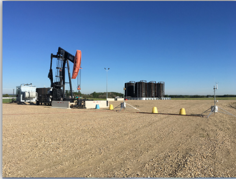
Figure 4. Sensor deployment at Site 8-8, showing the two sensor packages, the northernmost pump jack to the left, and the production tanks in the distance.
