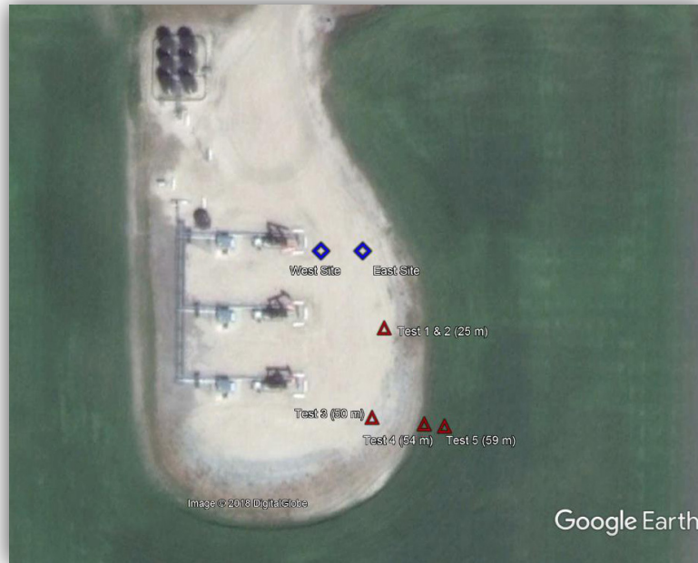
Figure 3. Map of Site 8-8 and sensor locations. Blue diamonds show the location of the methane sensors (East Site and West Site). Red triangles show where the controlled releases occurred.
