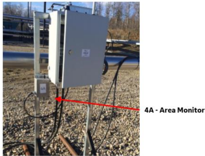
Figure 8.5-4 Far-Field LUMEN for General Area Monitoring of Methane Emissions
