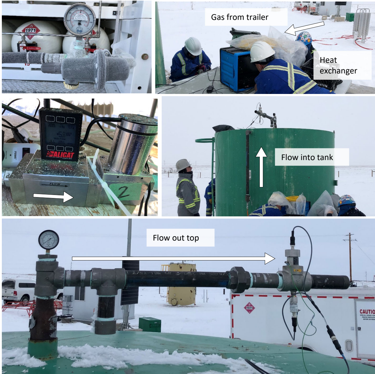
Figure 3: Flow Test Setup - Alicat Mass Flow Controller and 2-inch Ventsentinel® installed at CMC RI
