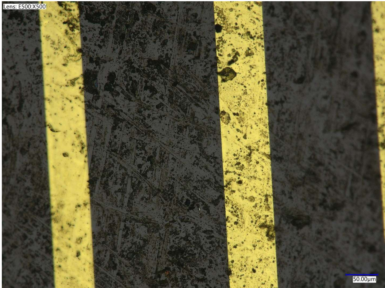
Figure 10: 500X magnification of top, thick conductors
