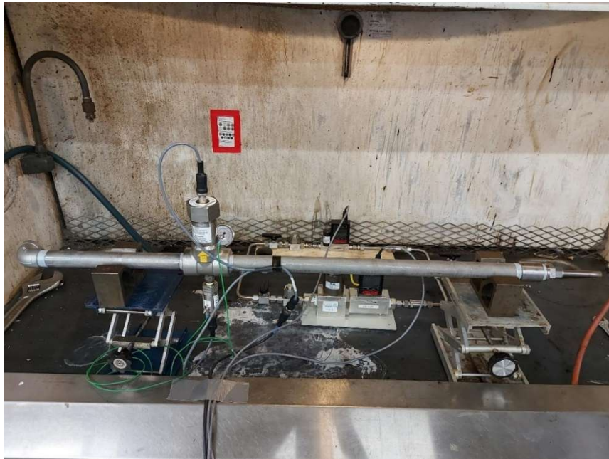
Figure 1: Flow test setup with two Alicat Mass Flow Controller and 1” Ventsentinel® installed in a fumehood.
