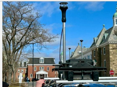
(Image of our vehicle-based hardware used in mobile methane measurement campaigns)
