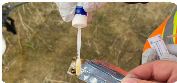
SLR Ecologists sampling a wetland for Canadian toad environmental DNA (eDNA) Credit - Megan Olson
