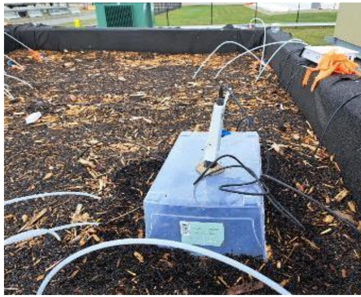
Static chamber used to measure surface fluxes of CO 2 using VAISALA VM-70 (CO 2 ) and CH 4 (SEM-5000)
