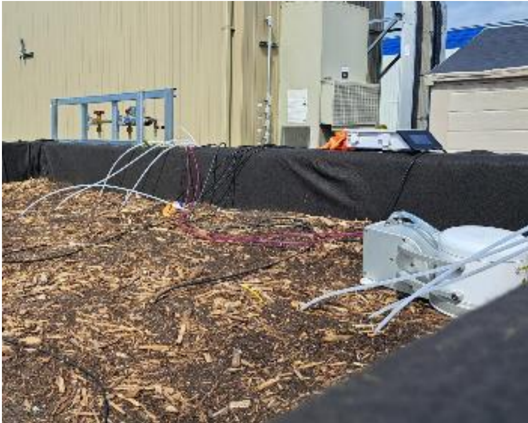
Automated EoSense CH 4 and CO 2 flux chamber
